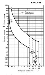
Trip characteristics: D Thermal trip 1.13...1.45 x I<sub>n</sub> Electromagnetic trip 10...20 x I<sub>n</sub> AC 15...30 x I<sub>n</sub> DC Calibration temperature 30°C
