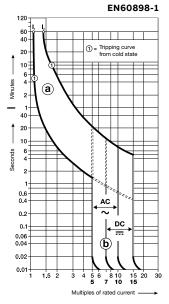
Trip characteristics: C Thermal trip 1.13...1.45 xl, acc. to EN60898-1 Thermal trip 1.05...1.3 xl, acc. to EN60947-2 Electromagnetic trip 5...10 xl, AC 7...14 xl, DC Calibration temperature 30°C
