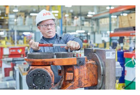
During Workshop Repair, your faulty parts are replaced by genuine Original Equipment Manufacturer (OEM) components. Following a rigorous repair, inspection and testing process, ABB ensure quality and reliability at lower cost.
