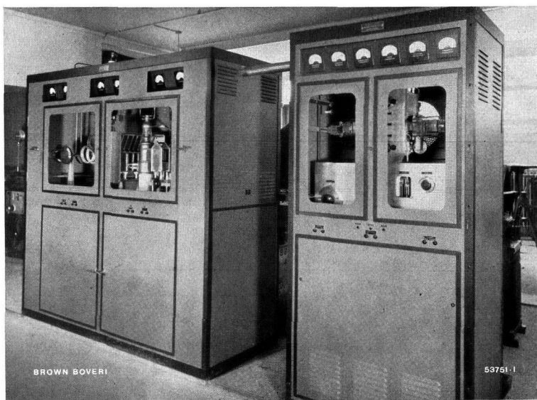
Fig. 12. — H. f. preliminary stages (right) and output stage (left). In the left-hand cabinet, a dismountable Brown Boveri transmitting tube can be seen, as well as parts of the anode oscillating circuit.
