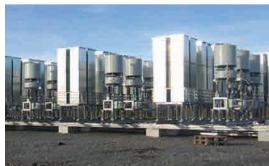
Figure 6. Cable simulator utilized during qualification of the Åsgard subsea gas compression system. Some flexibility included in the lumped components for different cable sizes and lengths.
