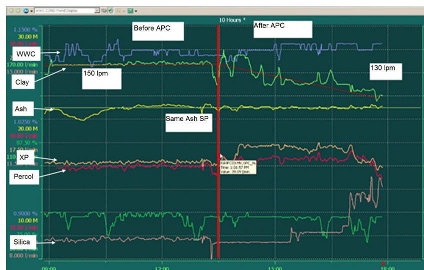
Figure 5. Performance comparison of paper ash (%) before and after 800xA APC Implementation
