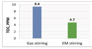
Figure 6. Total oxygen content in ball-bearing steel produced with gas and electromagnetic stirring respectively
