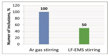
Figure 7 Number of non-metallic inclusions after EMS respective Ar gas stirring in the ladle furnace
