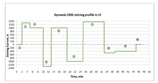
(1)before ladle arrival; (2)heat preparation; (3)slag building and alloying; (4)&(5)&(6)alloying and heating;
