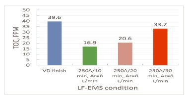
Figure. 4 The effect of soft EMGAS stirring time on the total oxygen removal in ladle refining
