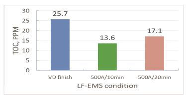
Figure. 5 The effect of EMS soft stirring time on the total oxygen removal in ladle refining
