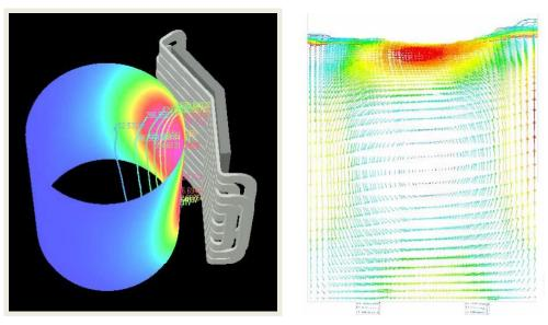
Figure 1. The 3D calculation of electromagnetic forces in a ladle installed with EMS (left) and the CFD velocity distribution in the melt (right)
