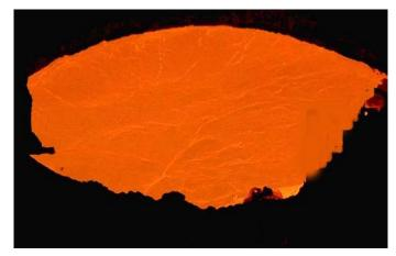
Figure 3. A slag open eye formed in the slag in a ladle surface with LF-EMS
