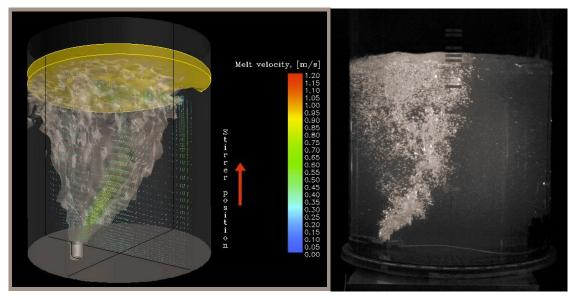
Figure 8. CFD simulation (left) and water modeling (right) results for EMGAS stirring in ladle furnace [11]
