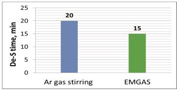
Figure 12. De-sulphurization time needed for sulfur reduction from 47 ppm to 7 ppm under Ar-gas and EMGAS stirring for a 150t ladle furnace
