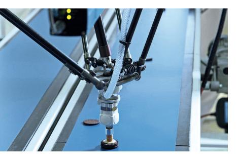
PickMaster application software with Generic Sensor Protocol, adds 3D vision technology to the ABB packaging application. It offers the ability to accurately locate and optionally inspect products of naturally varying size, height and shape such as bread, cookies, vegetables or meat both in the primary and secondary packaging stages.
