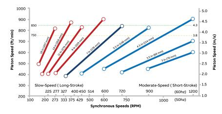
02 Ariel moderate-speed process compressors operate in comparable piston speed ranges to long-stroke, slow-speed compressors.
