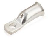
These lugs are designed with a narrow palm and are ideal for connecting to circuit breakers with limited terminal tunnel widths. The barrel of these lugs are designed as per the Australian Barrel Scheme hence the same crimping rules apply. The barrel entry has a bell-mouth design to ease cable insertion, specially when using fine stranded (flexible) cable.
