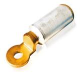
These lugs are used to terminate Aluminium conductors to Copper termination points. They are made from 99.9% pure copper palm and 99.6% pure aluminium barrel, friction-welded together for a strong and highly conductive electrical joint. Each lug is individually packaged and comes capped with jointing compound pre-filled inside the barrel ready for use. These lugs are crimped using dies compatible with Aluminium barrels.
