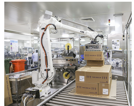
An IRB 4600 robot is at the heart of the unique packaging system.
