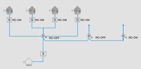
Looping through gateway as auxiliary power supply. Each distributor is connected to branching into 4 lines with each. Each line looping through the building gateway.
