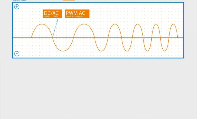
The drive calculates the motor's required voltage and current. DC power is then fed into an inverter producing AC power at the precise voltage and current needed.
