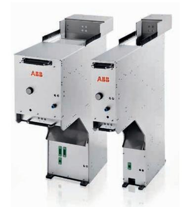
systems. Driven by pneumatic cylinders, the FlexFeeder takes parts from an unordered bulk supply and dispenses them in small quantities onto the flat picking surface in the field of view of the robot's vision system. Sensors detect when the tank needs to be refilled. The tank can be purged without power
