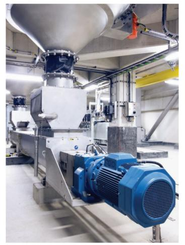
ABB's low voltage IEC process performance motors, from 3.0 to 22.0 kW, were selected for the screw conveyor project. Here the motor is packaged with a Dodge in-line helical Quantis reducer.
