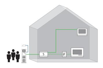
IP-gateway enables the wireless remote use of the door entry system.
