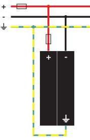
Figure 1: Installation of MMP C100PV & MMP C550PV Protectors.
