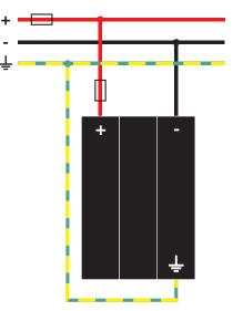
Figure 2: Installation of MMP C1000PV Protector.
