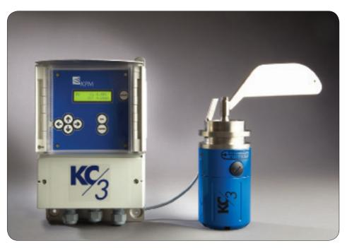
KC/3 Blade Consistency Transmitter has two main sensing blade types, standard for 2-8% process consistency and MC for 6-16% process consistency.
