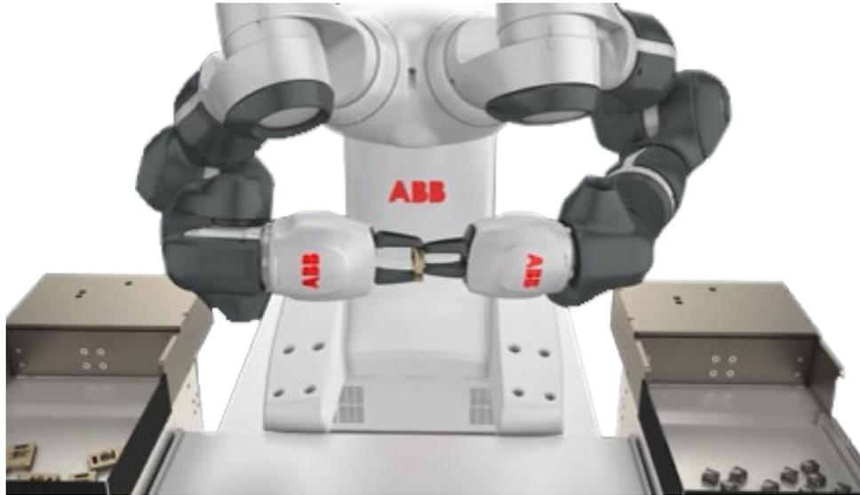
YuMi working side-by-side handing finished parts to be packed.
