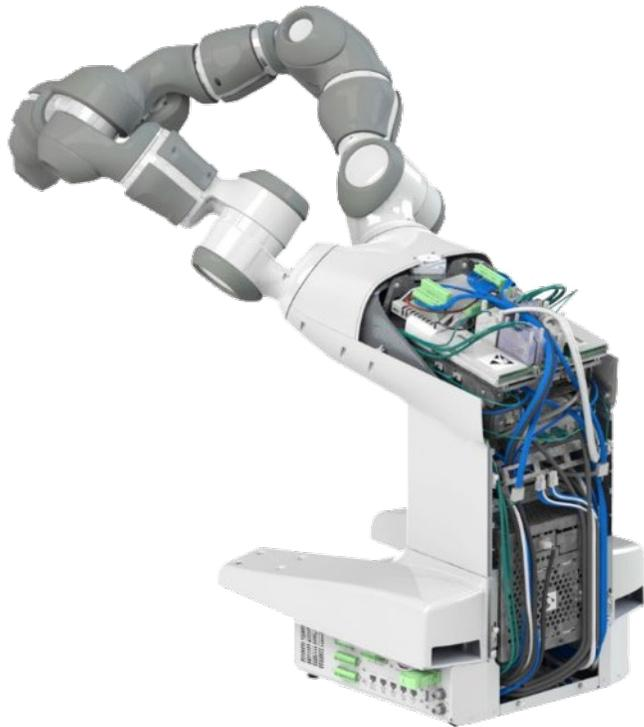
Embedded controller based on IRC5
