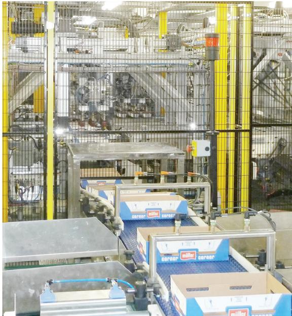
The functional requirement of the repack system was to take packed yogurt from a pallet, produce a multi pack, repack and palletise.
