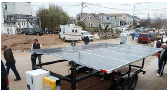
Chris Mejia of Consolidated Solar and Shaun Chapman of SolarCity help set up a 10-kilowatt solar generator on Staten Island.
