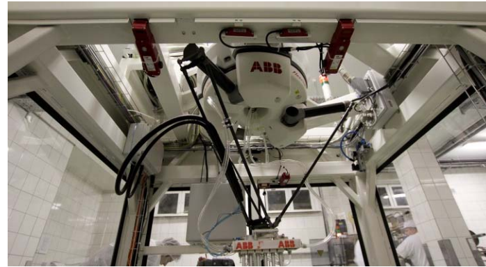
450 PPM capacity per robot
