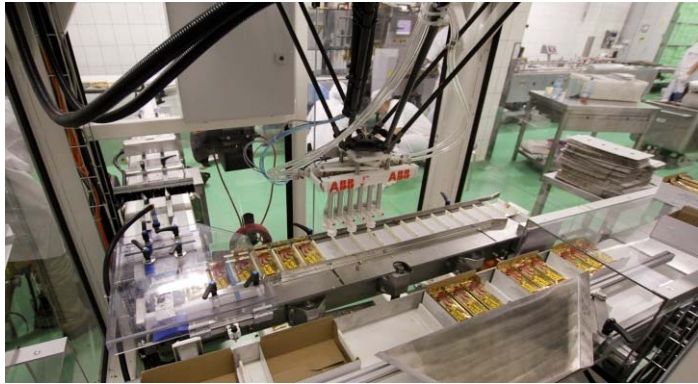
Indexing belt with small footprint
