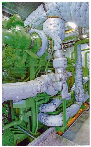
Power2 two stage turbocharging on the test beds at ABB Turbocharging in Baden, Switzerland
