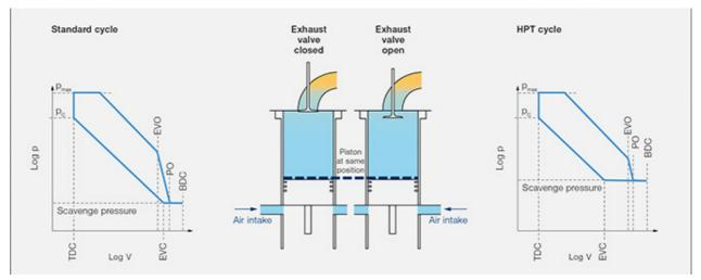
Fig. 2: Standard versus HPT cycle
