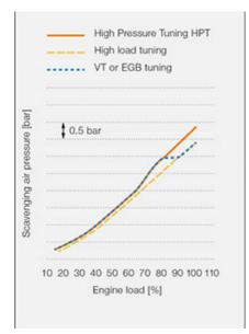
Fig. 1: Scavenging air pressure tuning curve
