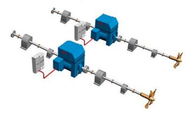
Figure 1: Overall principle of the shaftinstalled electrical auxiliary propulsion system. The propulsion drive including the brake resistor (A) is fed from the auxiliary generator. The feeder may require a transformer to match the voltages. The drive feeds the auxiliary propulsion motor (B) when the main propulsion engine is disconnected from the shaft.
