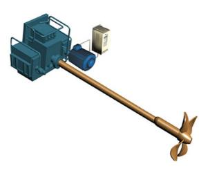
Figure 4: Overall principle of the gear-installed electrical auxiliary propulsion system. The propulsion drive including the brake resistor (C) is fed from the auxiliary generator (D). The drive feeds the auxiliary propulsion motor (B) when the main propulsion engine is clutched from the shaft. The gear ratio of the reduction gear (A) allows for smaller and lighter motor sizes than possible in direct installations.
