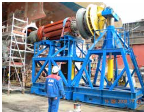
Servicing the Azipods on a cruise ship
