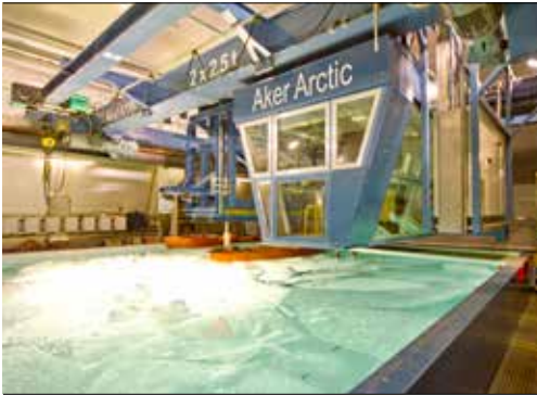
The Aker Arctic ice lab test models in scale 1:25
