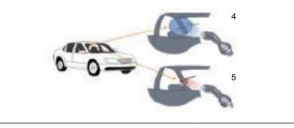
1 Pattern Control Function, Dual SA Structure<sup>-1</sup> | 2 Small Pattern for Narrow Area | 3 Large Pattern for Wide Area | 4 Wide pattern wasted paint | 5 Controlled pattern conserved paint
