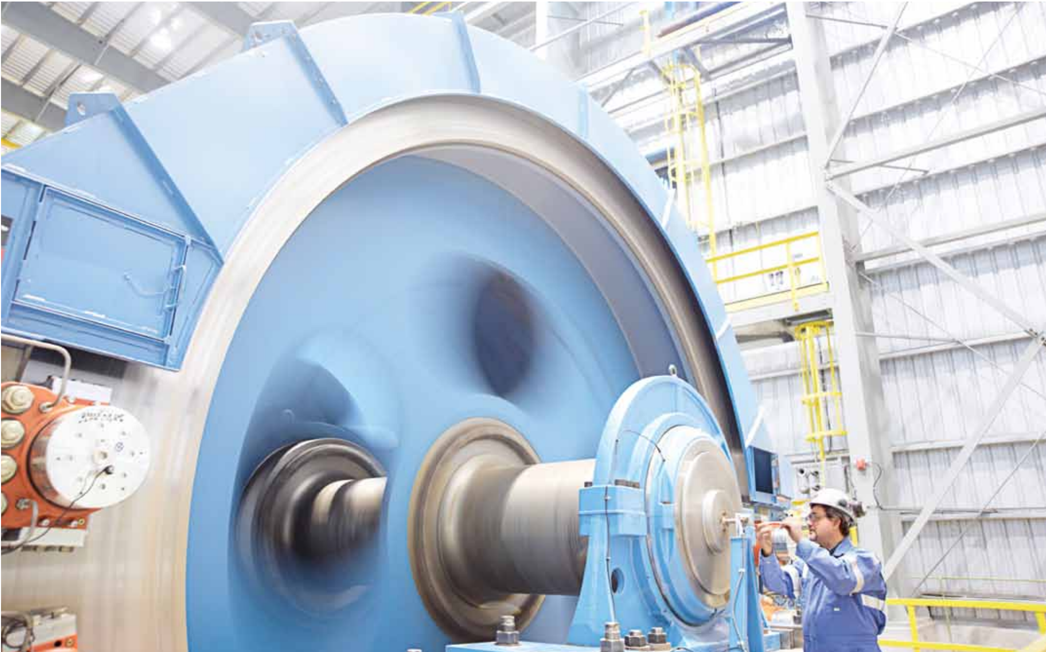
Mechanical hoist drum at Totten mine, Sudbury, Ontario, Canada – equipped with energy-efficient drives from ABB
