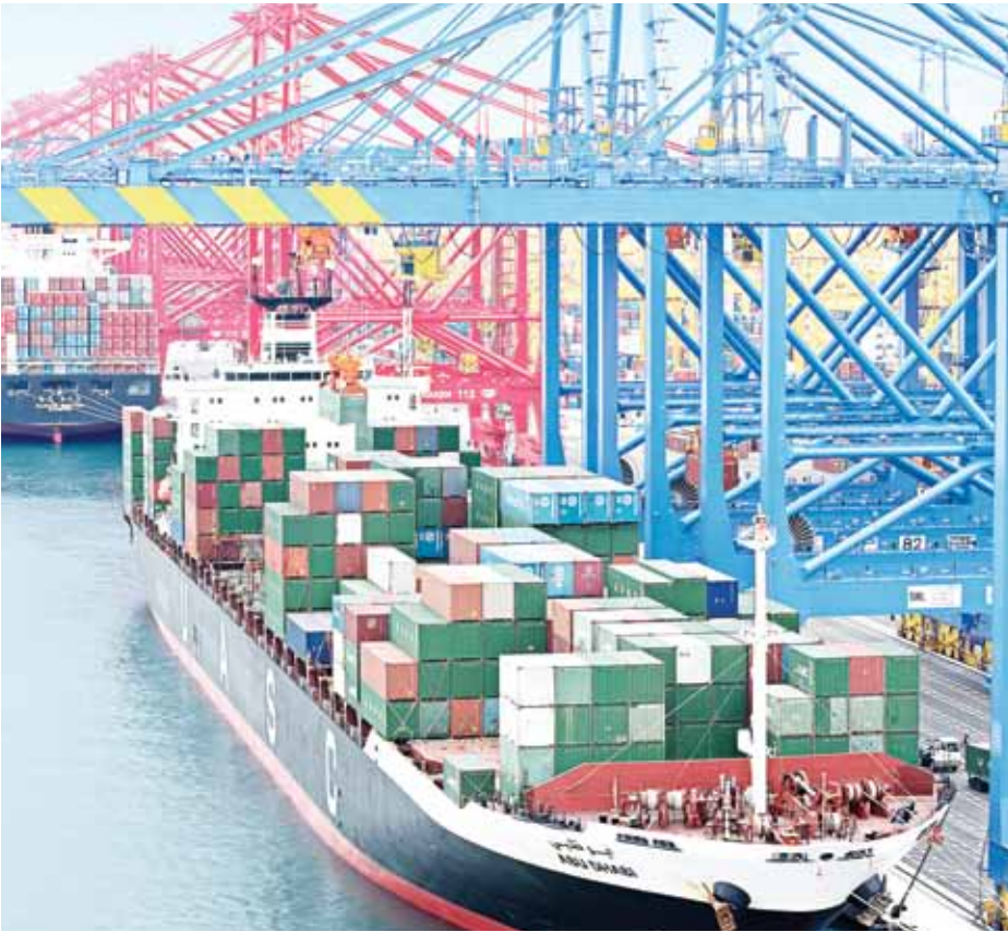
Dual hoist ship-to-shore cranes – Busan, South Korea
