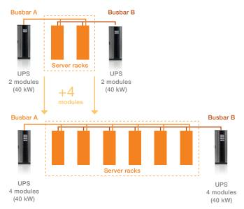
The power demand in the sample configuration increases from 40 kW (N+1) to 120 kW (N+1). The UPS is perfectly capable of adapting to this increase in power demand.
