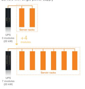
In this distributed power protection concept, the power demand grows from 40 kW (N+1) to 120 kW (N+1). The UPS can be easily adapted to meet the power demands of the growing infrastructure by adding four 20 kW modules.
