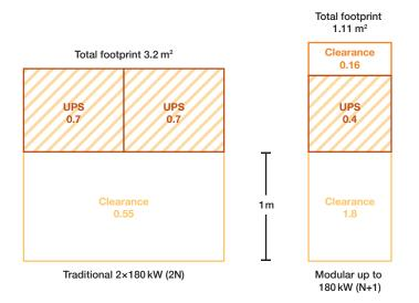
Modularity minimizes space requirements and maximizes predictability of future space requirements. In the example shown,  $2 m^2$  is saved.
