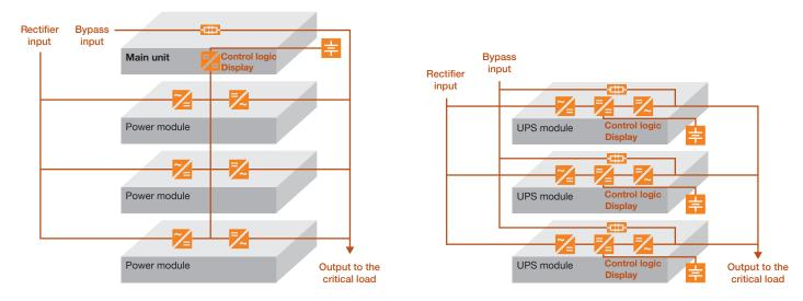
Modular UPS with common system components
