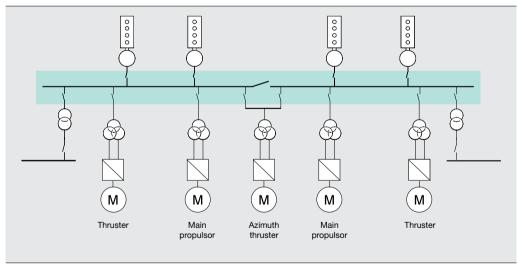
Reduced fuel consumption in an electric propulsion system can be attributed to two key elements. The first is the variable speed control of the propeller, which reduces the "no-load" losses of the propellers to a minimum compared with classical fixed-speed controllable-pitch propellers. The second element is the automatic start and stop of the diesel engines, which ensures that the engine load is kept as close to its optimum operating point as possible, within the limits of operation.
