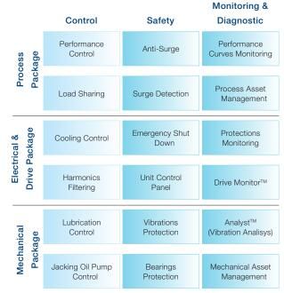
Example of DEIC packages setup for VSD-driven pipeline compressor
