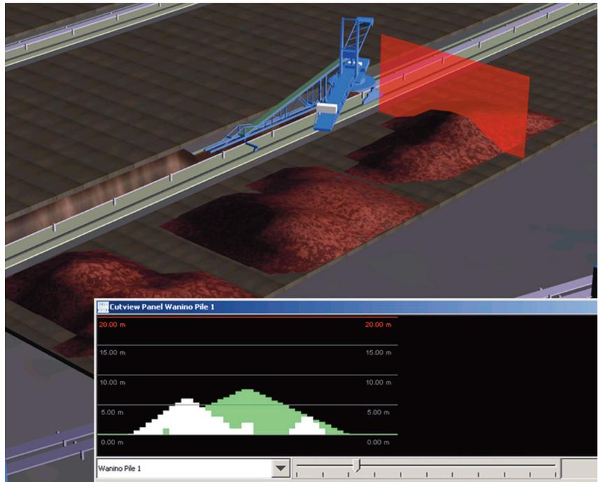
Figure 5. Selection of a cut view.
