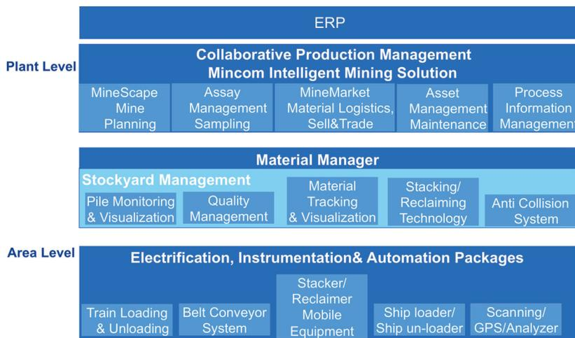
Figure 2. Modular system for bulk material handling.
