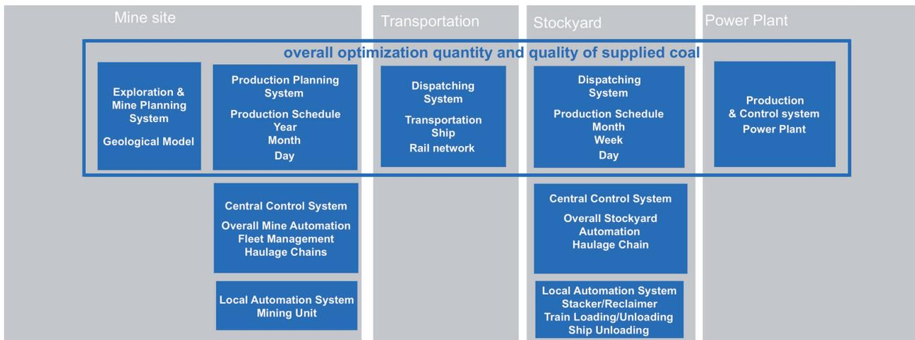
Figure 1. Integrated coal management system.
