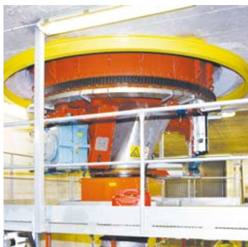
VFD driven screw application with torque sensing for feeding fuel out of residual storage.
