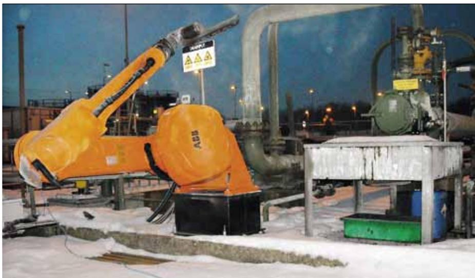
The ABB and Shell demonstrator has shown that robots can be used in oil and gas facilities to perform high precision operations in all kinds of weather.
