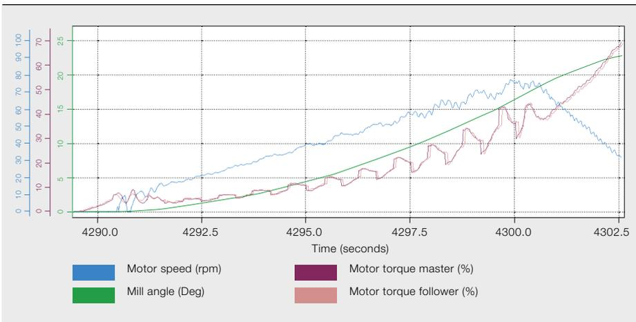
Even during the frozen-charge remover function sequence, in which torque steps are applied to the system to loosen frozen material in the mill, the torque of the slave perfectly matches that of the master drive system with no obvious signs of oscillations or backlash → 6. Backlash would be seen by a drop in torque to zero or even negative values, but since torque and speed are always positive, backlash does not occur.
