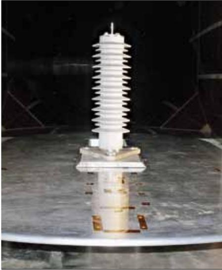
100m/s. The danger of a significant reduction of the creepage distance caused by deformation of the arrester housing can therefore be ruled out.
