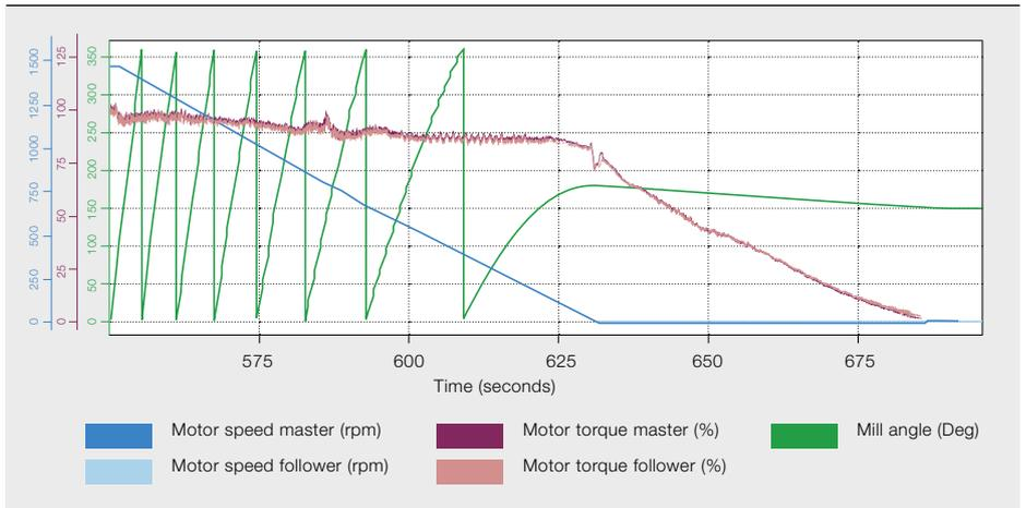
hold the mill with the charge unbalanced. By slightly reducing the torque, the mill rolls gently back until the charge is balanced. Because the torque is always positive, even when the direction of rotation of the mill changes and during controlled rollback, contact is always maintained between the teeth of the two pinions and the ring gear, thereby ensuring no backlash can occur.
