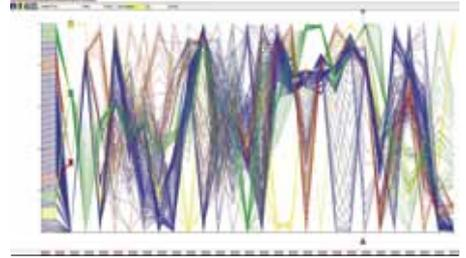
this data is used to create the benchmark model. Current process variable values are compared to this benchmark model to determine whether the current data is within or outside of this normal operation.
