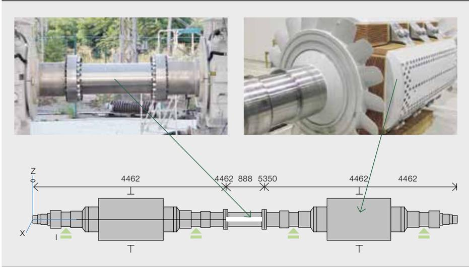
The back to back test arrangement makes it possible to run the ASDs at their rated power, a condition not otherwise possible during either the compressor string test nor during site test.
