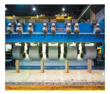
applied by concentric rings. On the other side of the sheet is a unique optical (confocal) measurement. The confocal measurement is combined with a magnetic reference measurement, and the result is caliper measurement. The simplicity of this design provides reliable performance day after day in the harsh paper mill environment.
