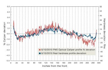
Figure 1 – Profile correlation between Optical Caliper and handheld hardness instrument
