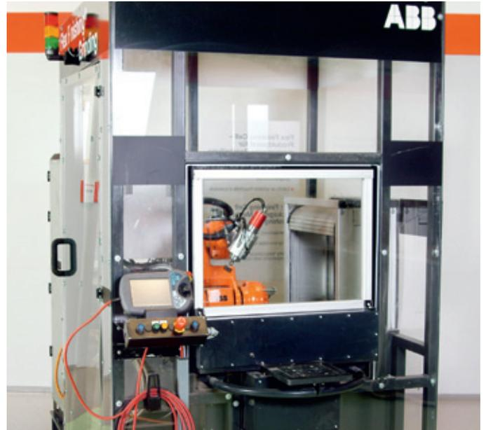
The Flex Finishing Cell represents a standardized, verified robot solution in the form of a robotized cell, which can be programmed for different tools and adapted to different components and work objects.
