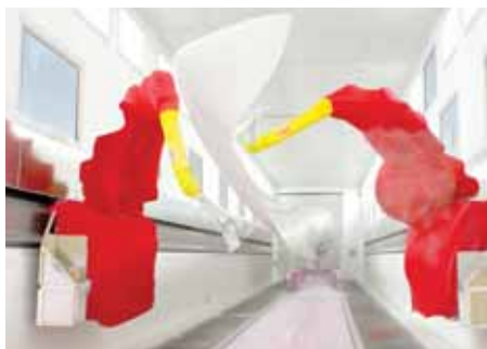
ABB robots painting a wind turbine
