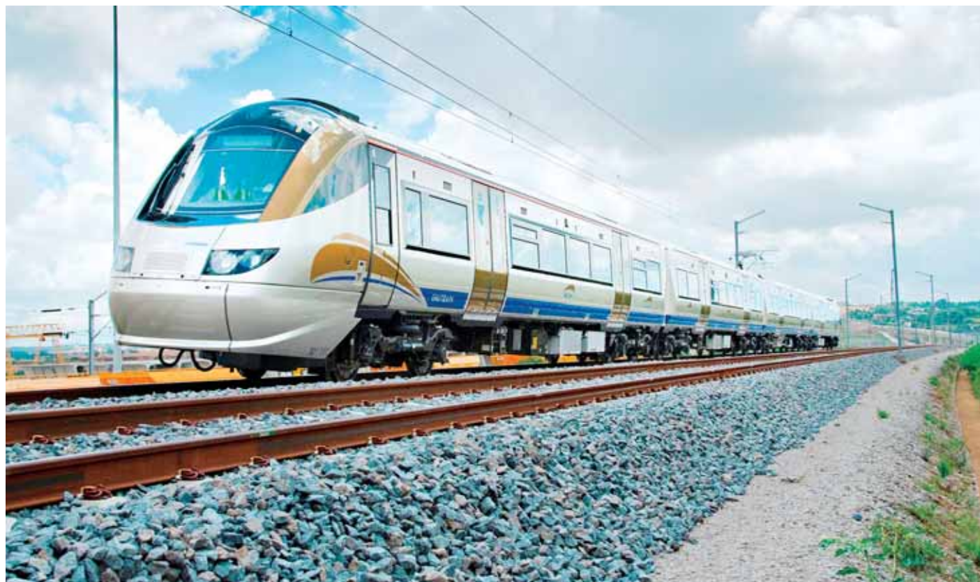
Gautrain is a variant of Bombardier's hugely successful Electrostar, all 1,600 cars of which are powered by ABB traction transformers and motors
