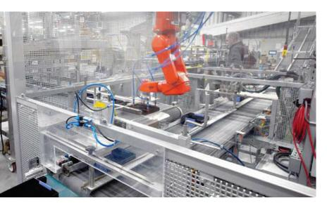
When BDMO automated the final stage of its production process for Vivabox packaging, the production speed went up 20-35 percent.
