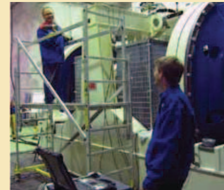
Figure 5: Testing is teamwork. Matti Tervonen from ABB Marine prepares to give the test rig a blow with impact hammer to measure its modal characteristics, while Aki Kinnunen from VTT is ready to record the results.
