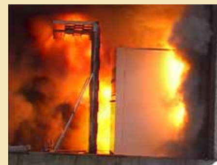
Figure 4: Internal arc testing of MV switchboard, from NEF1 High Power Laboratory
