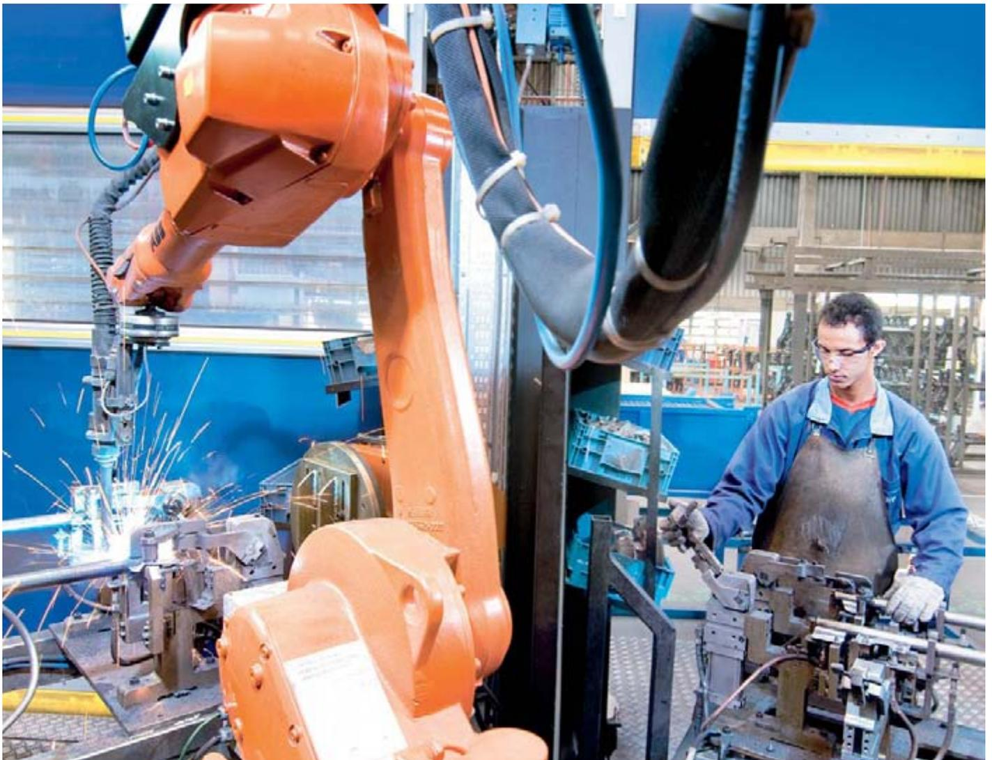
**A**t Benteler Automotive in Brazil an ABB IRB 1600 robot is attaching mounting clips to door beams destined for use in Toyota Corolla cars. In the time it takes a factory worker to load two pillars, each with five clips, into one side of the welding station, on the other side the robot is surely and quickly executing seven welds per pillar. Operator and robot switch sides, and the process is repeated – over and over again, 24 hours a day.
