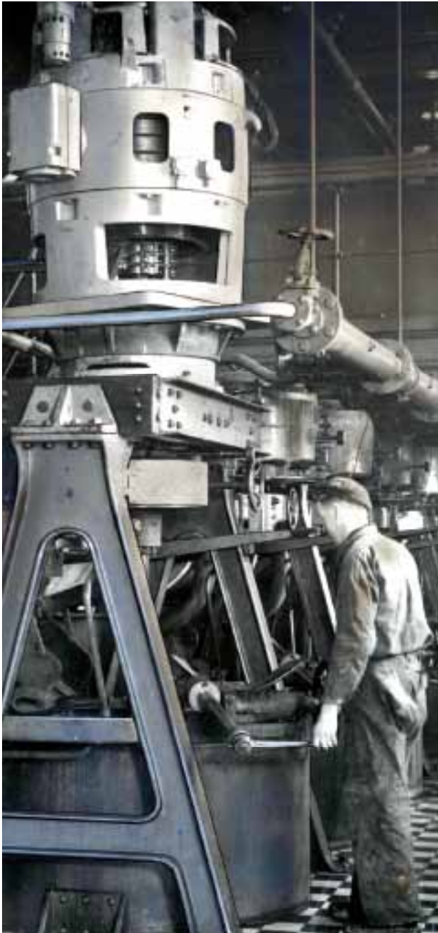
Fully automatic power system for operating sugar centrifuges in 1943
