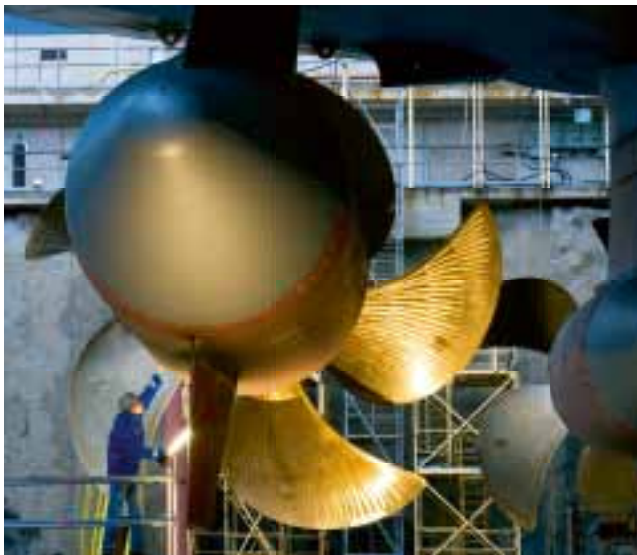
An Azipod unit in dry dock, 2009. The pod contains the high-efficiency electric motor that drives the propeller, saving space on board for additional cargo and greater design flexibility.
