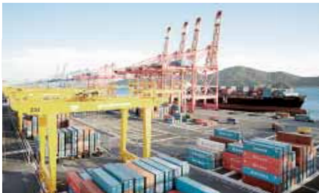
Dual-hoist, ship-to-shore cranes and automated rail-mounted gantry cranes at Busan Newport in South Korea, installed by ABB in 2009.
