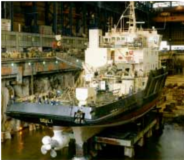
Waterway service vessel Seili was fitted with the first Azipod prototype in 1990. Azipod propulsion has now been installed in 81 vessels and has accumulated more than 5 million hours of operation.
