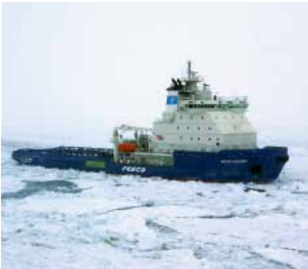
Icebreaking support vessel Fesco Sakhalin uses two 6.5 MW Azipod units, delivered 2006. ABB is the world's leading supplier of power and propulsion systems for the marine industry.
