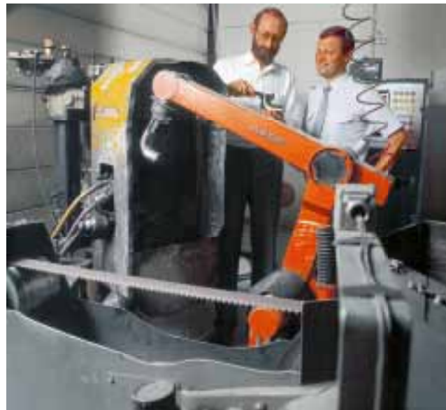
In 1974, Magnusson AB became Asea's first external robotics customer. The company used the robot to polish stainless steel pipes for use in the food industry.
