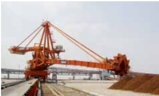
Automated cranes were installed by ABB in 2009, modernizing Shanghai's Luojing port, China's largest bulk-cargo terminal. ABB's electric crane systems are three to four times more energy efficient than diesel cranes and produce no local greenhouse gas emissions.
