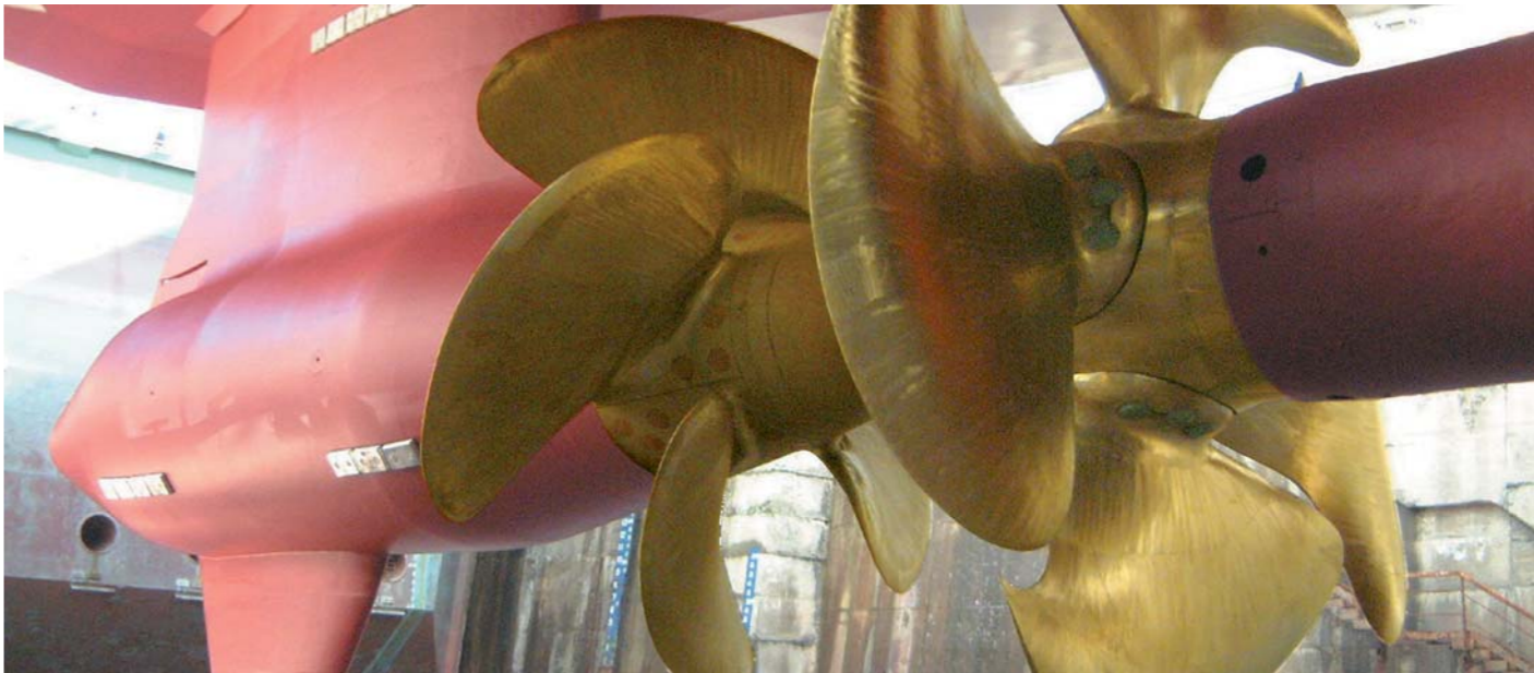
Shown above is an Azipod® unit used in a contra-rotating propulsion (CRP) solution.
