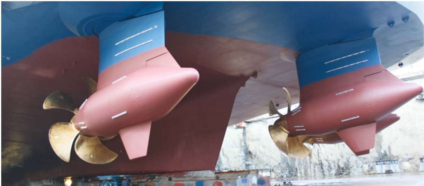
Oasis of the Seas was built at STX Europe, Turku shipyard, with a triple Azipod® propulsion solution.
