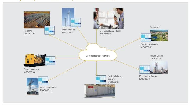
sets of controllers exchange information with each other in real time. Based on the load levels of the fossil fuel generators, the MGC600-P automatically adjusts the set point and enables the generators to run at their optimal load, while ensuring the maximum amount of renewable energy is utilized by the microgrid.
