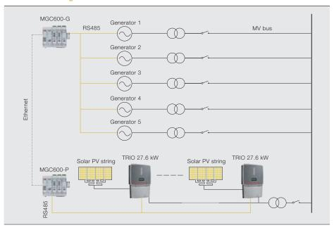
MGC600 controllers are the building blocks of the Microgrid Plus System.
