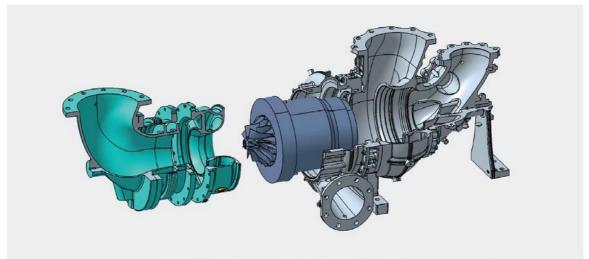
is no need to remove the insulation of the turbocharger anymore, since only the flange connection of the air inlet needs to be accessed during service (Fig. 5).
