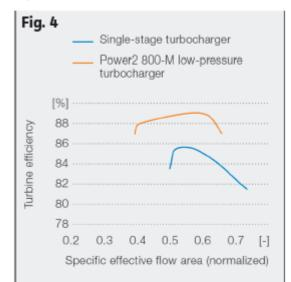
**Fig. 4:** Turbine efficiency vs. specific effective flow area of a single-stage turbocharger and Power2 800-M low-pressure turbocharger.
