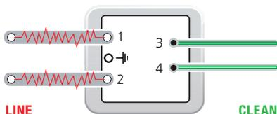
All dirty (line) incoming tracks are separated from the clean output tracks, individual line and clean tracks are routed close together. Earth pins are bonded to an earth layer/plane.
