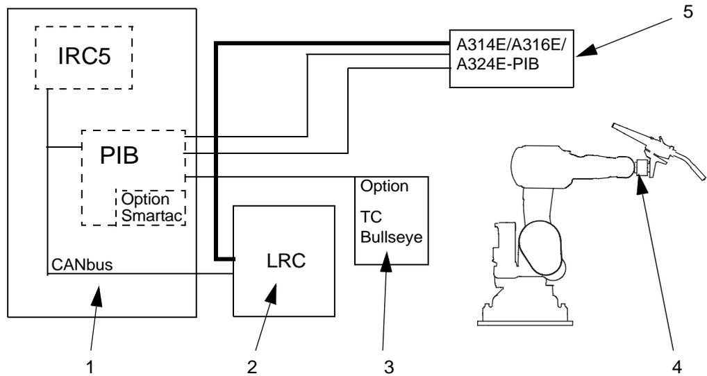
Figure 2. Overview of “ARCITEC” connections LRC 430
