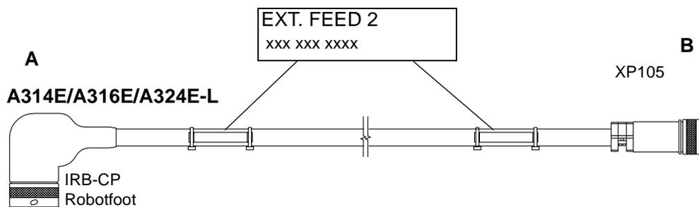
Figure 17. Feeder cable 2, A314E/A316E/A324E-L.
