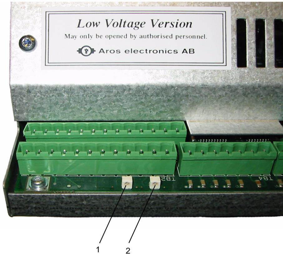
Figure 38. Light-emitting diodes on PIB
