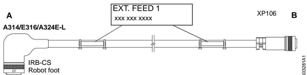
Figure 15. Feeder cable 1, A314E/A316E/A324E-L.
