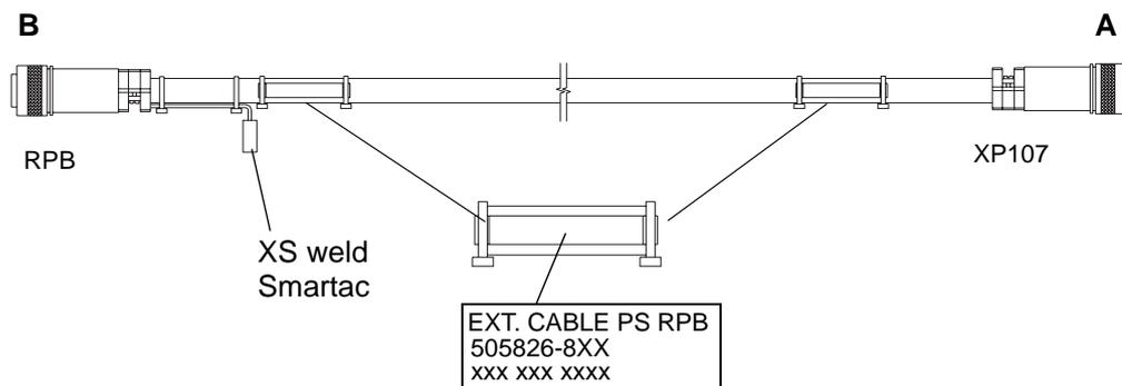
Figure 21. Control cable RPB
