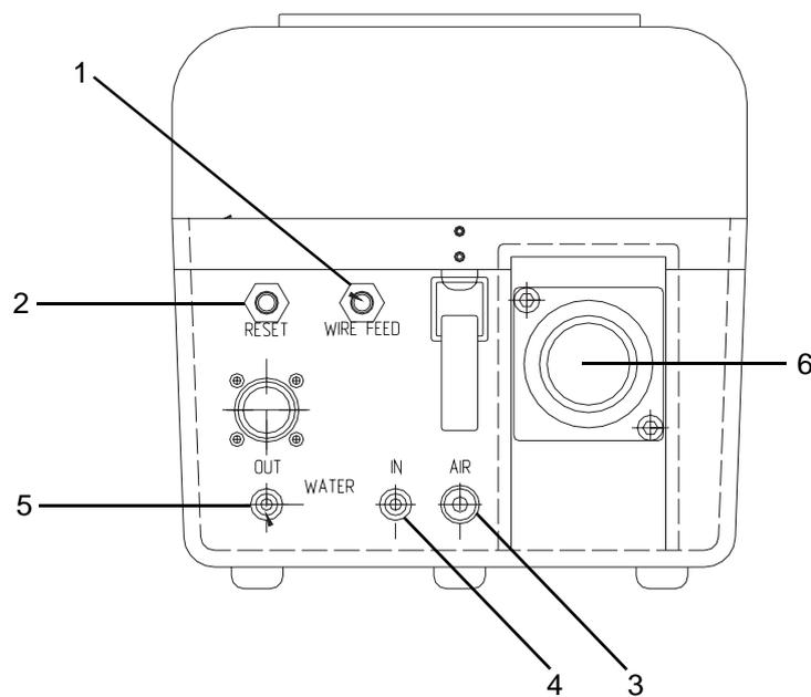
Figure 7. Side of the wire feed unit.
