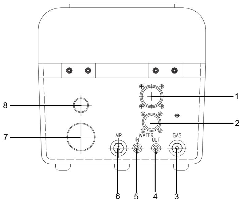
Figure 12. Connections on wire feed unit
