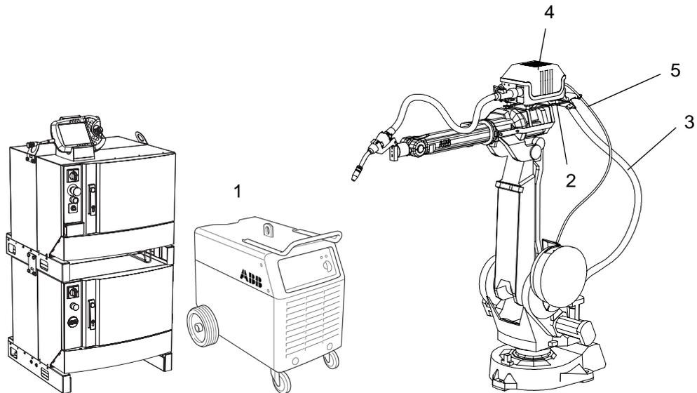
Figure 5. IRB 2400 with welding equipment
