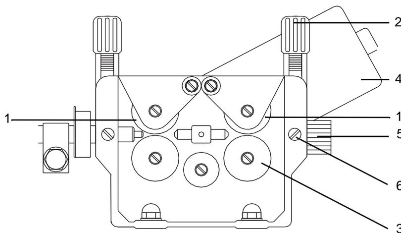
Figure 28. Wire feed unit
