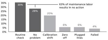
Potential for predictive maintenance with pressure transmitters. Source Shell Global Solutions
