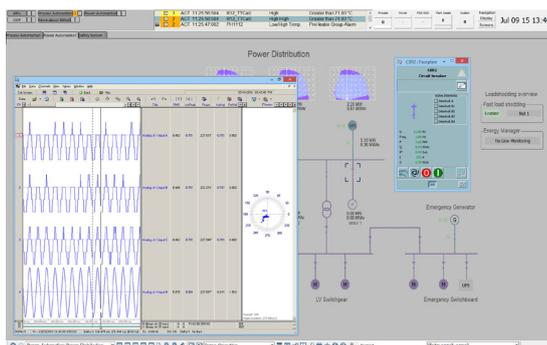
Change parameterization for all protection relays through the web interface directly from system 800xA.
