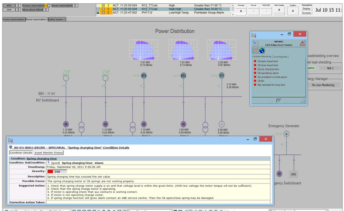
“In a stress situation, for example, power failure on an incoming cable, we can go into the automation system and reconnect the entire 6.35-kV switchgear from pre-programmed sequences,” [...] “We know what needs to be done and then the system knows the order in which it will happen. No need to run in front of the cabinets and control the switches.” — Arne Jönsson, electrical manager at Kemira Kemi
