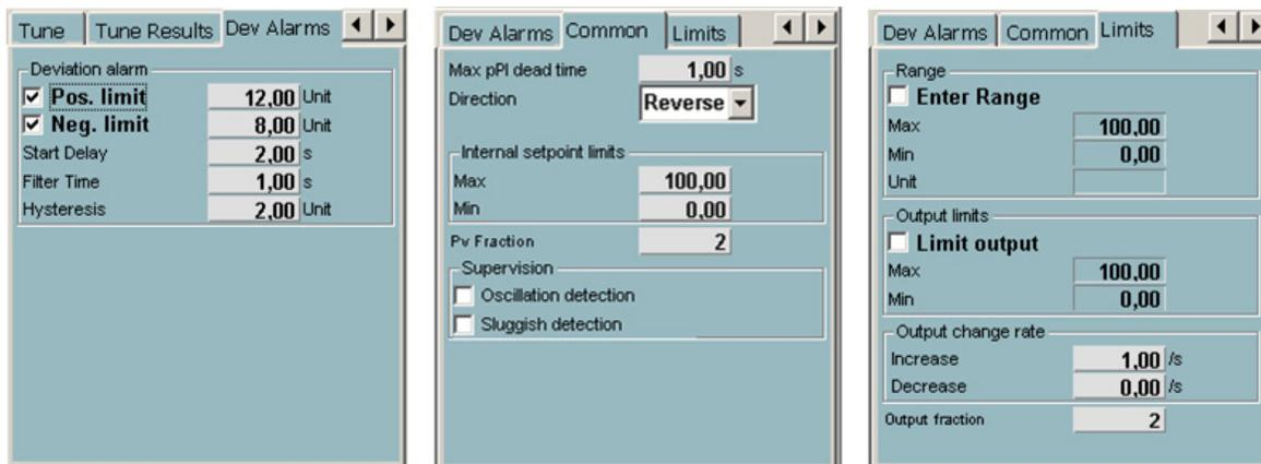
Figure 49. The settings of deviation alarms, common and limit settings in a PidAdvancedCC control module
