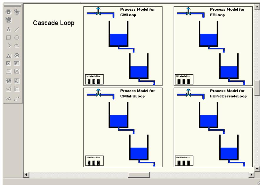
Figure 146. The Cascade Loop application in online mode showing four methods of programming
