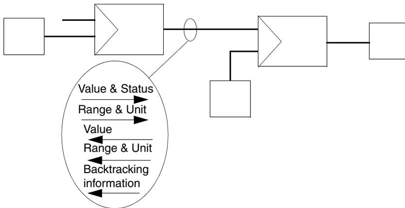
Figure 32. A graphical connection of ControlConnection type with its main signal flow forward and a flow backward
