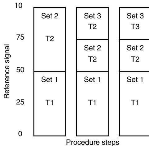
Figure 92. Example of the procedure for gain scheduling in three sets
