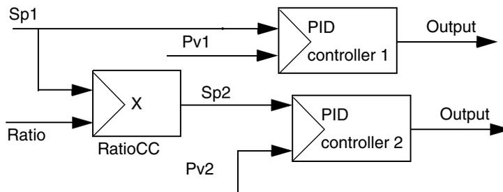
Figure 55. Example of ratio controllers where the setpoint from the first controller is multiplied by a factor to obtain the setpoint for the second controller
