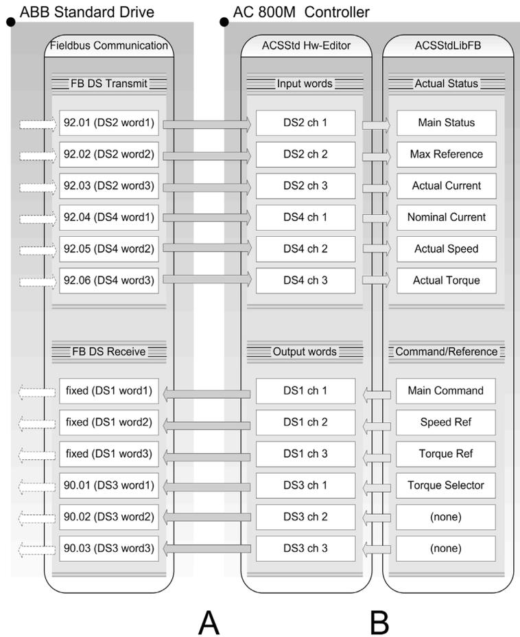
Figure 191. Overview of the connections between an ABB Standard Drive and an AC 800M Controller, part A-B
