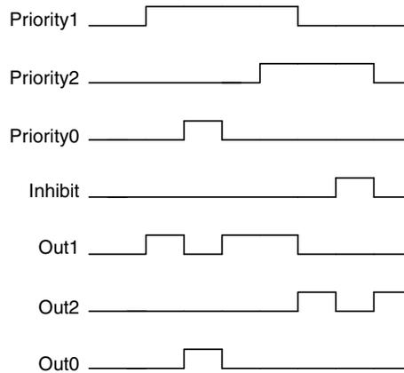
Figure 159. State diagram showing Priority command priorities and output signals with the effect of Inhibit
