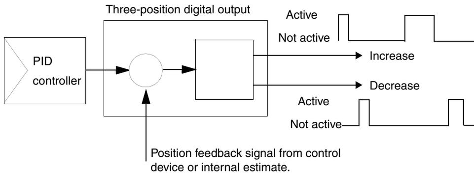
Figure 94. The principle of the three-position digital output function
