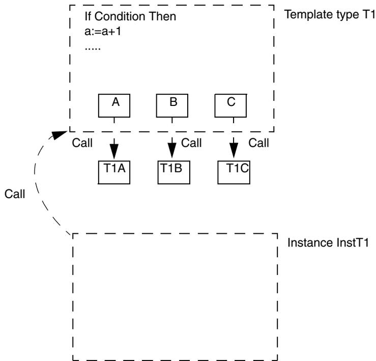
Figure 22. Execution of an instance of a template type with formal instances
