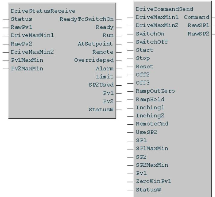
DriveStatusReceive are used to retrieve the status from a drive, after which the program or operator makes a decision based on this information. A command can then be issued to the drive using DriveCommandSend.
