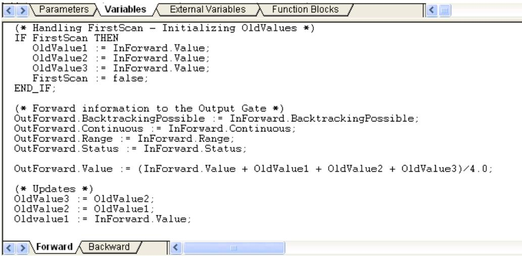
Figure 67. Programming code in the Forward code block
