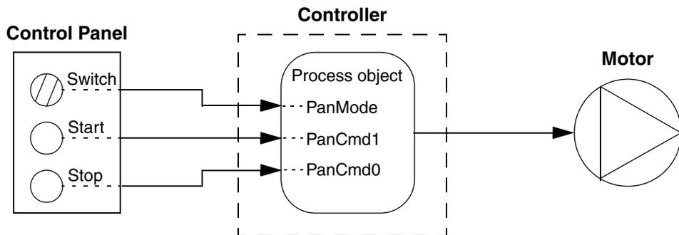
Figure 187. Control steps in Panel mode. This solution is recommended for small applications, where all three panel parameters are connected from a control panel
