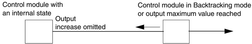
Figure 31. Example of when a succeeding control module has reached a limit value; the preceding control module stops further integration (anti-windup)
