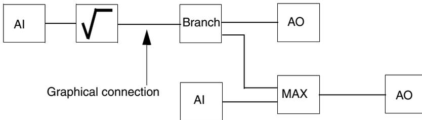
Figure 29. A chain of connected control modules for analog signal handling
