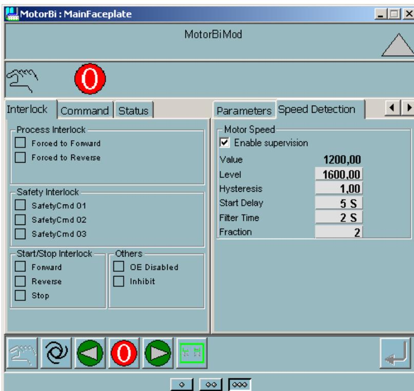
Figure 257. MainFacePlate of the MotorBiMod type in online mode
