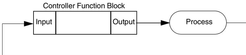
Figure 52. A control loop defined by a function block
