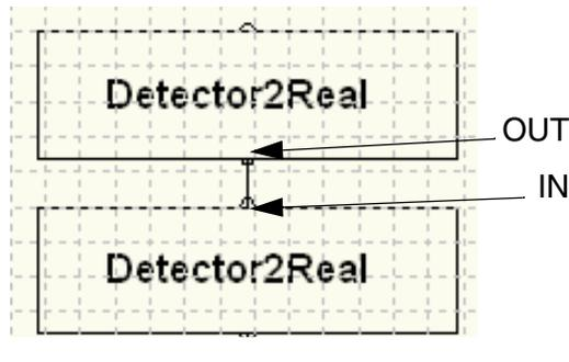
Figure 224. A graphical connection to the next Detector2Real module
