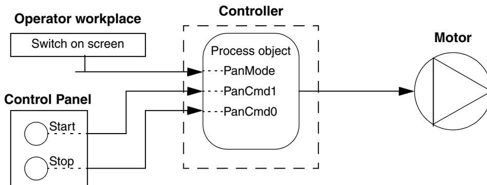
Figure 188. Control steps in Panel mode. This solution is recommended for large applications, where the *PanMode* parameter is connected to an operator workplace
