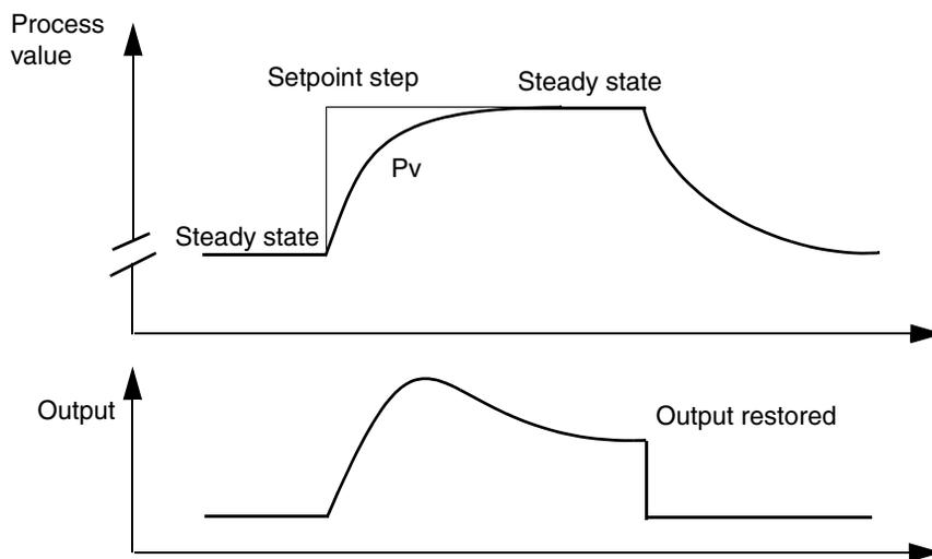
Figure 88. Setpoint step identification and output restoration
