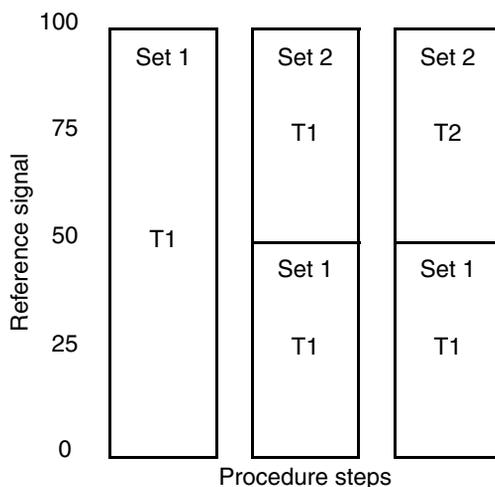
Figure 91. Example of the procedure for gain scheduling in two sets
