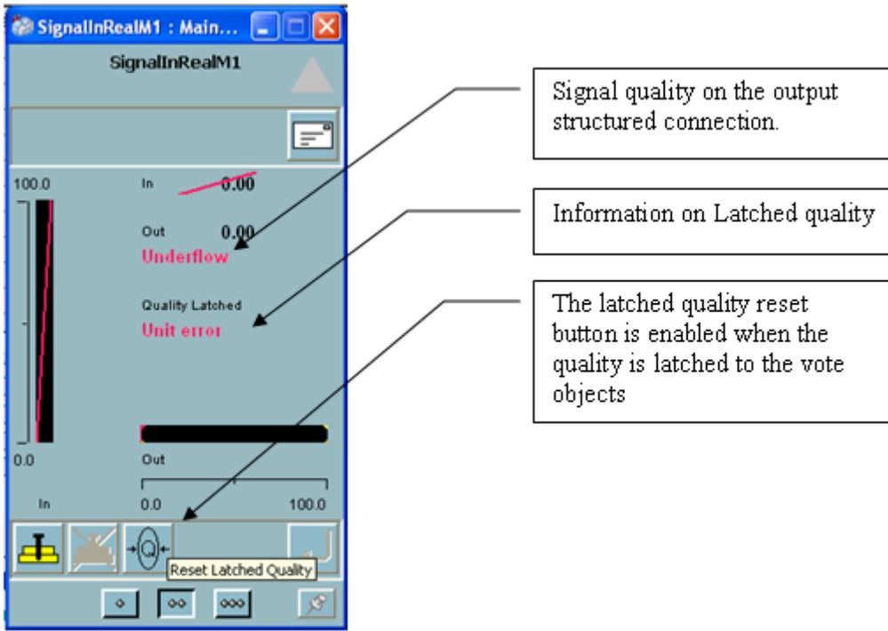
Figure 216. Latched information on a real input signal object
