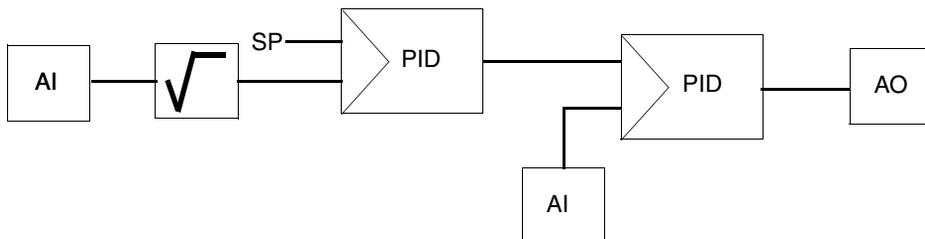
Figure 28. Example of graphical connections between control modules making a control loop
