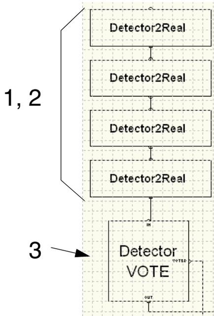
Figure 221. The four Gas detectors and a connected Vote module presented in the CMD Editor in FireAreaFA11
