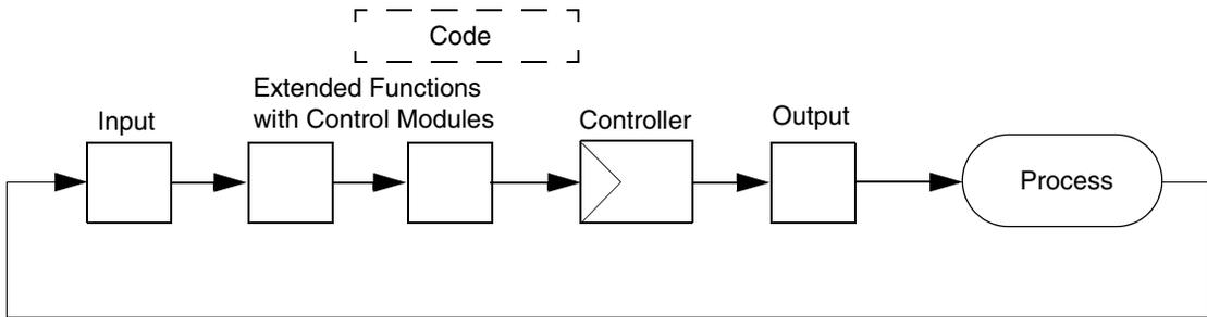
Figure 51. A control loop with all functions defined by control modules from the control libraries
