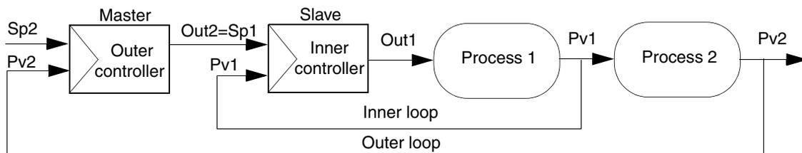
Figure 53. Illustration of two controller modules connected in cascade
