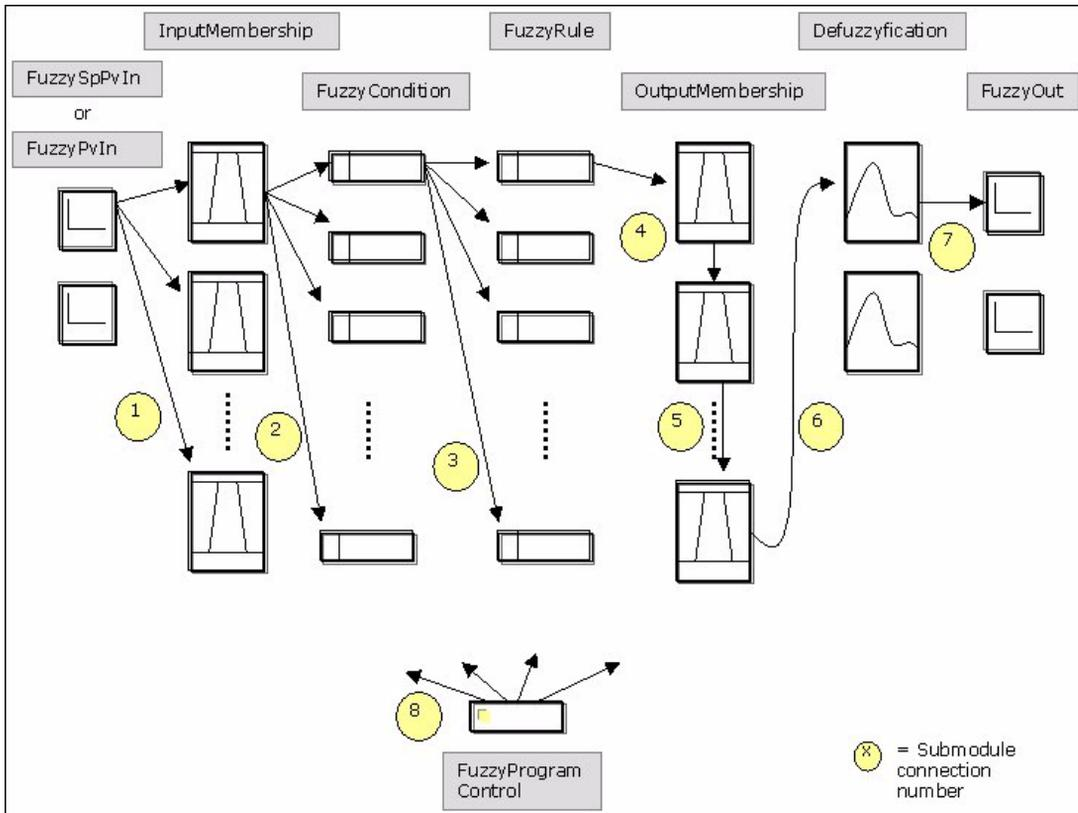
Figure 45. Sub-module connections in the fuzzy controller templates
