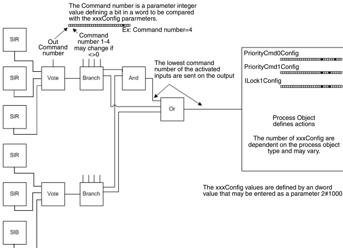
Figure 205. Configuration example of vote logic. (SIR=Signal In Real, and SIB=Signal In Bool)
