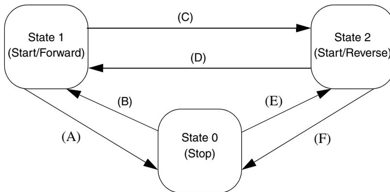
Figure 158. Manual maneuvers interlocking signals
