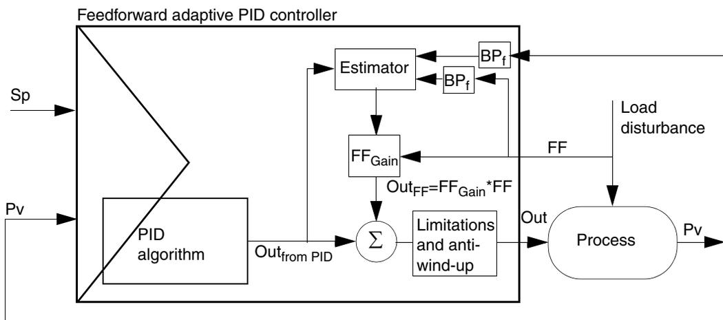
Figure 90. The principle of the feedforward adaptive PID controller
