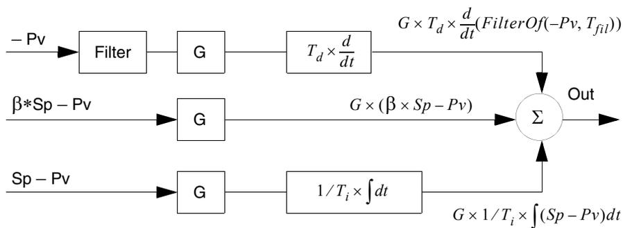
Figure 36. The principle of an ideal PID controller
