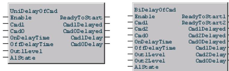
If, for example, a level detector informs an object to start, a disturbance pulse should not be able to start the object. The object shall not start until the detector delivers a reliable, constant signal stating that the start level is reached. If the object is a motor, this behavior is very important, in order not to wear it out.
