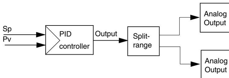
Figure 56. Example of split-range control where the output range from the controller is divided into two branches with different ranges
