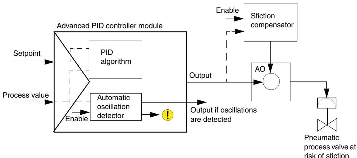
Figure 95. Principles for detecting and solving friction problems
