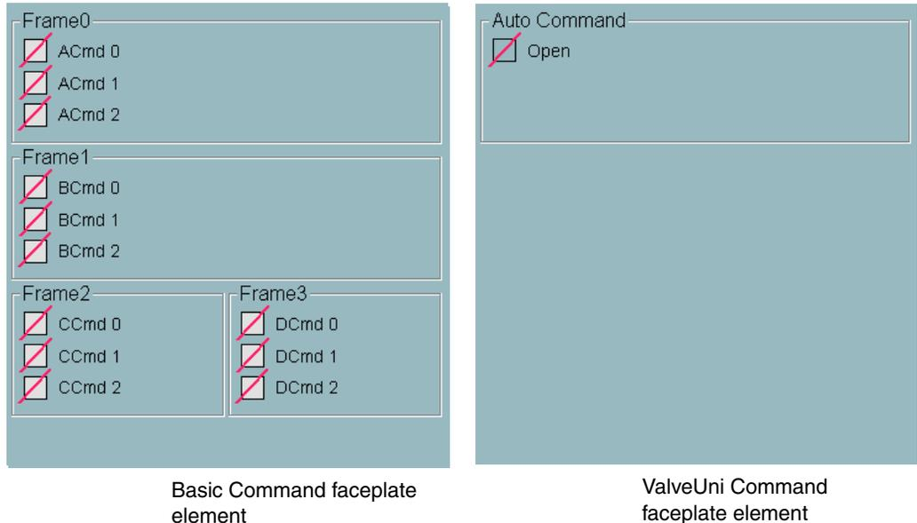
Figure 173. The basic Command faceplate element and the corresponding one in the ValveUni(M) type
