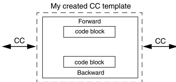
Figure 57. A control module prepared with two code blocks for handling forward and backward directions
