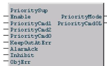
It can be used, together with the OEText function blocks, to generate error messages.
