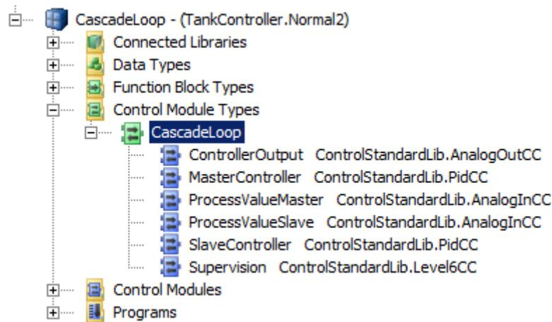
Figure 10. Cascade loop in Control Builder
