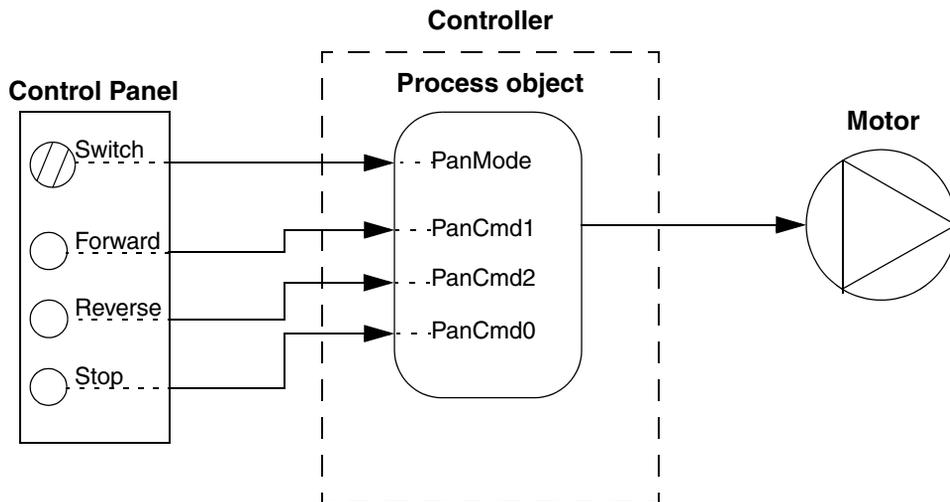
Figure 189. The Panel mode control diagram. A general solution for smaller applications, where all four Panel parameters are connected from a control panel
