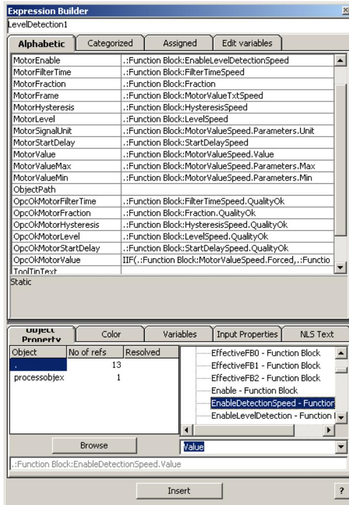
Figure 182. All the connections have been made to the LevelDetectionSpeed in the Expression Builder
