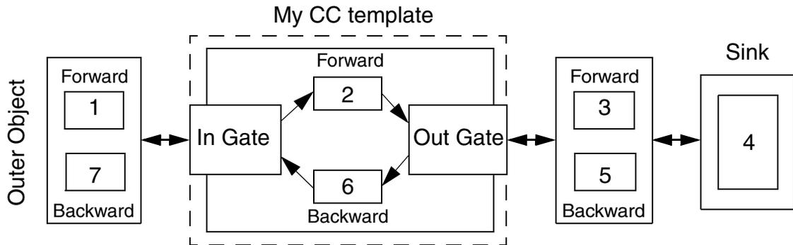
Figure 61. My CC template object is protected by the Gate modules on both sides to ensure a secure signal traffic with ControlConnection
