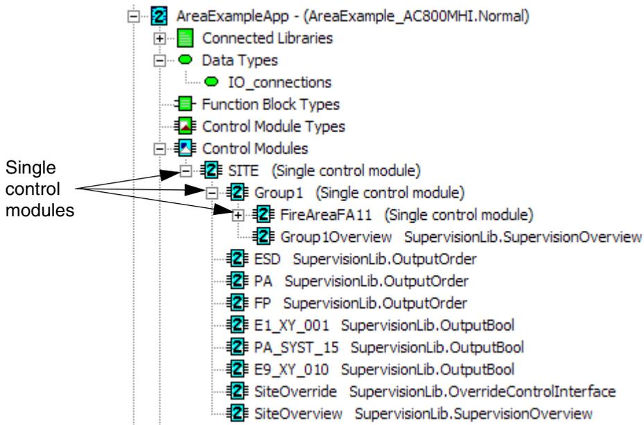
Figure 217. The single control modules represents each level display
