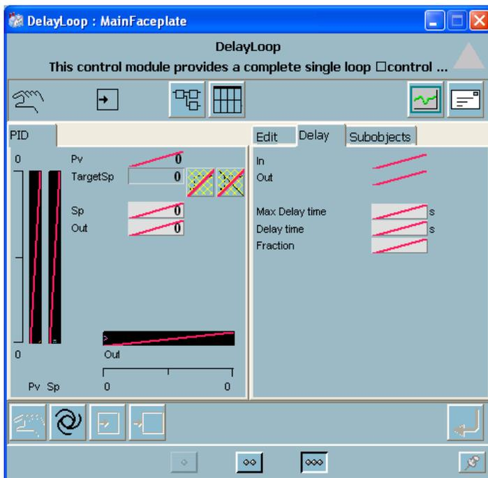
Figure 126. Extended Faceplate of DelayLoop
