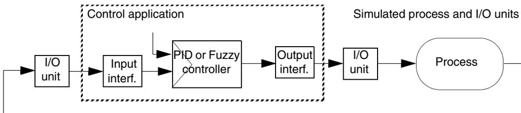
*Figure 143. The principle for control applications, the simulated processes and I/O units*
