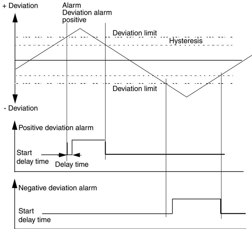
Figure 84. Overview of the controller deviation alarm limits
