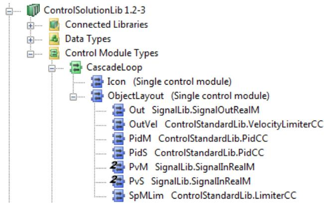
Figure 105. Standard types in a control loop solution (*CascadeLoop*)
