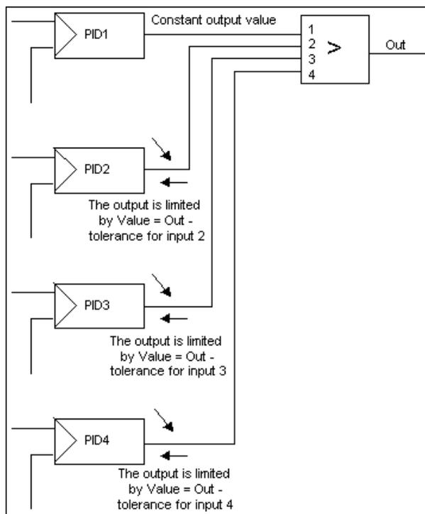
Figure 137. Example of a Max4CC control module with inputs from controller outputs
