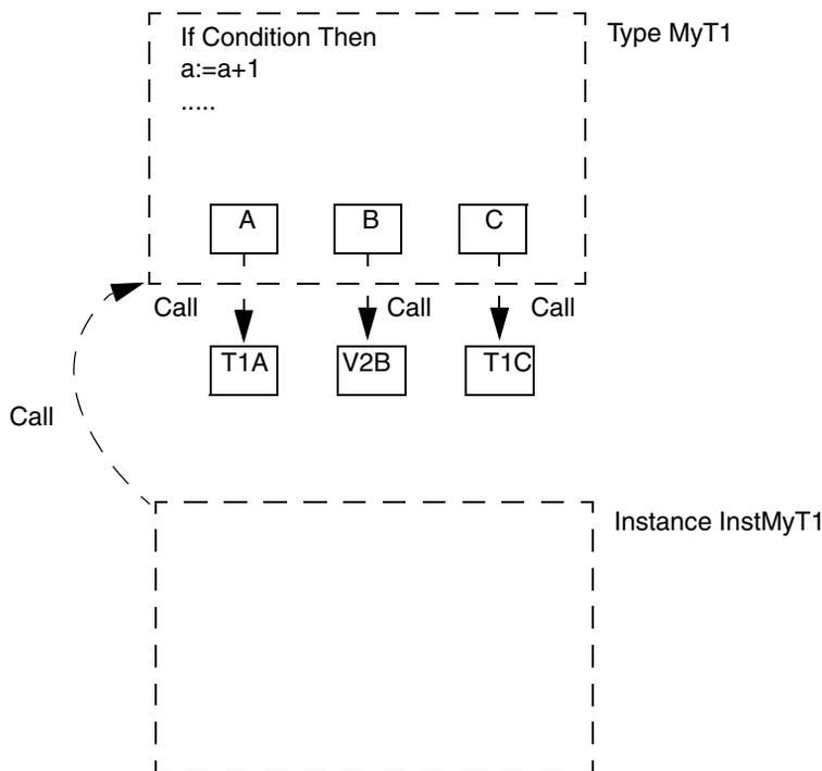
Figure 26. Execution of an instance of a modified template type copy
