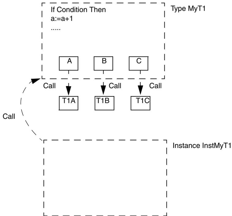
*Figure 24. Execution of an object based on a template type copy*
