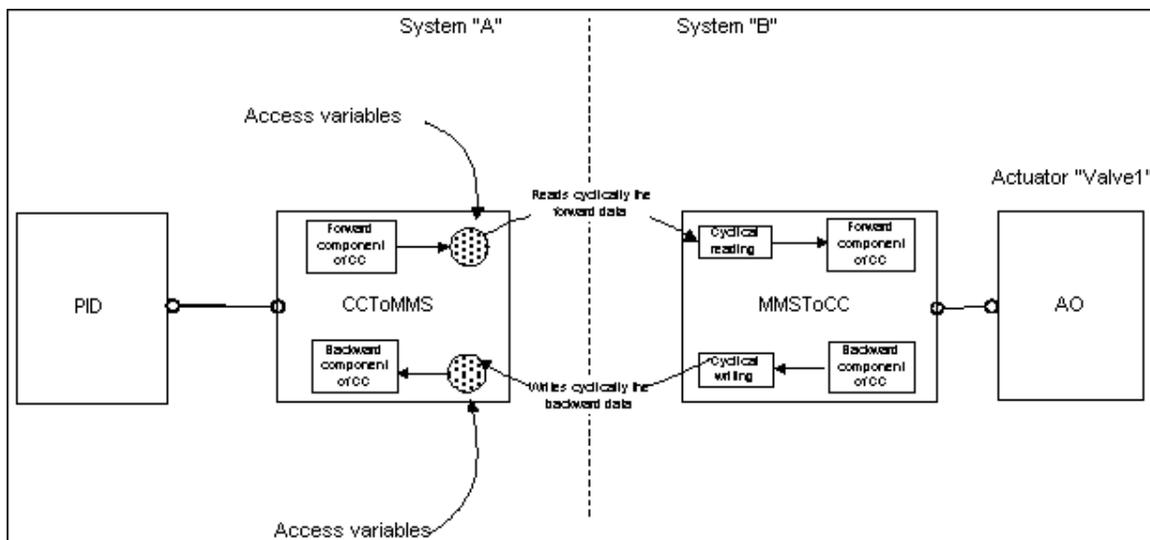
Figure 33. ControlConnection using control modules
