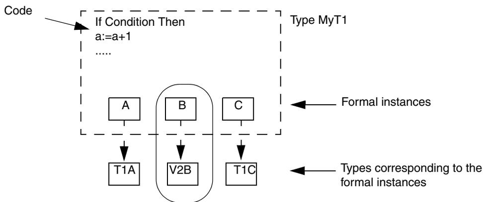
Figure 25. Copy of template type with formal instances, modified by replacing one of the formal instances (circled in the figure)
