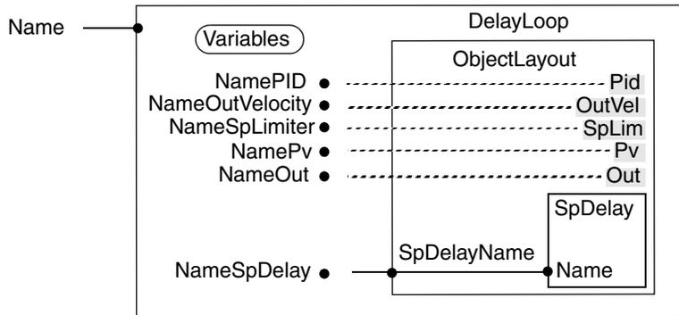
Figure 119. The result of DelayLoop parameter and variable connections
