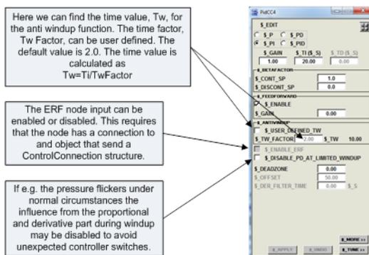
Figure 40. The EDIT interaction window of a PidCC or PidAdvancedCC
