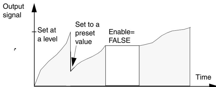
Figure 103. The integrator function sums the input signal ( $In$ ) value over time
