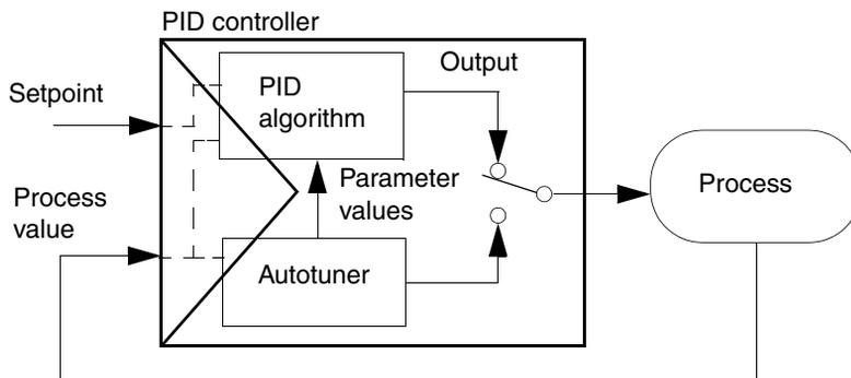
*Figure 86. The principle of autotuning in a PID controller with the Autotuner function*
