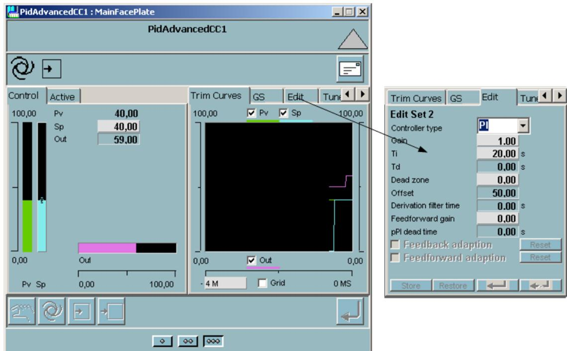
Figure 46. The extended faceplate for the PidAdvancedCC control module with trim curves and parameter settings
