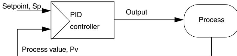
Figure 34. A control loop with the function block of a PID controller
