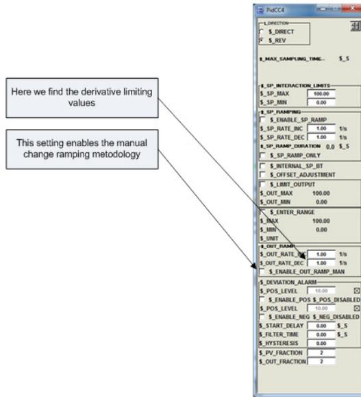
Figure 41. The interaction window of a PidCC or PidAdvancedCC
