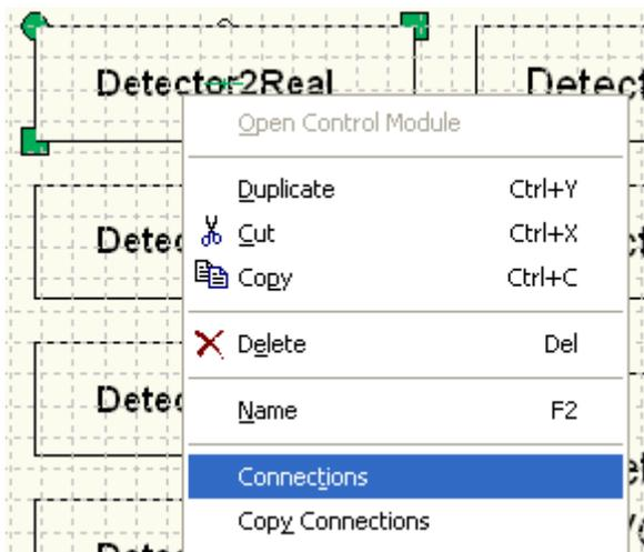
*Figure 222. Open the connection editor for the first gas detector module*
