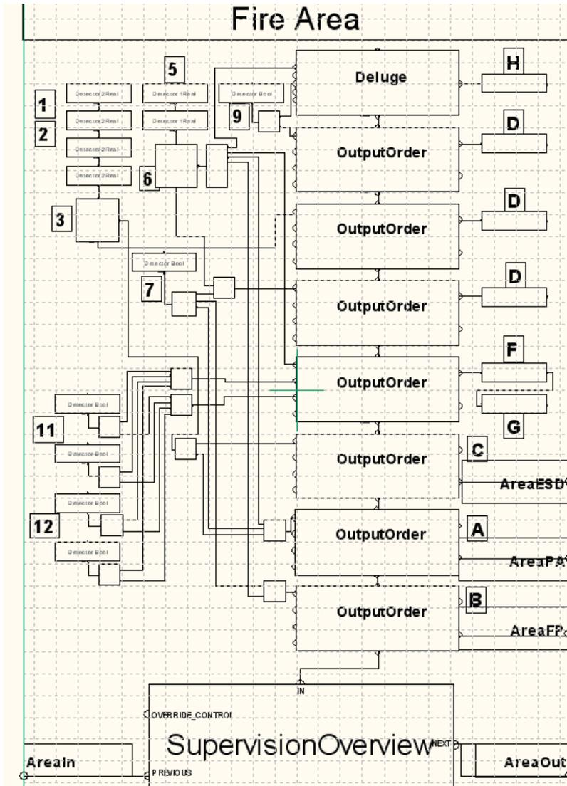
Figure 219. The FireAreaFA11 in the CMD Editor, with letters and numbers corresponding to the fire protection data sheet
