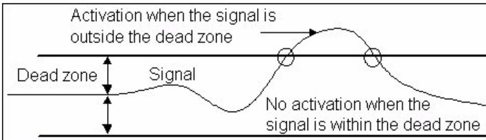
Figure 39. A dead zone on both sides of a desired signal value
