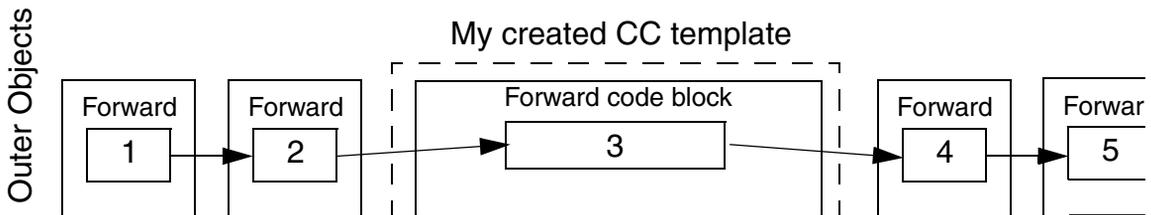
*Figure 58. ControlConnection will always start with forward block (1), and then execute forward block (2), your forward block (3) and then (4), (5) etc.*
