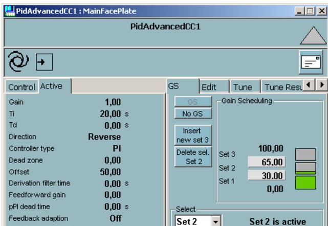
Figure 47. PidAdvancedCC control module with gain scheduling (GS) when Set 2 is active
