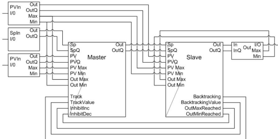
Figure 135. Example of a cascade control loop consisting of function blocks, with signal ranges added
