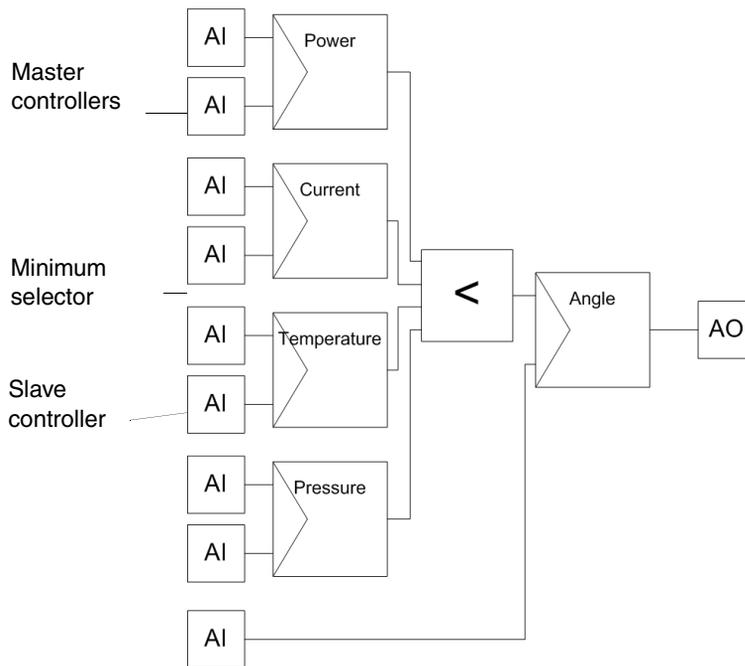
*Figure 138. Example using control modules for override control in a heat pump using a minimum selector control module*
