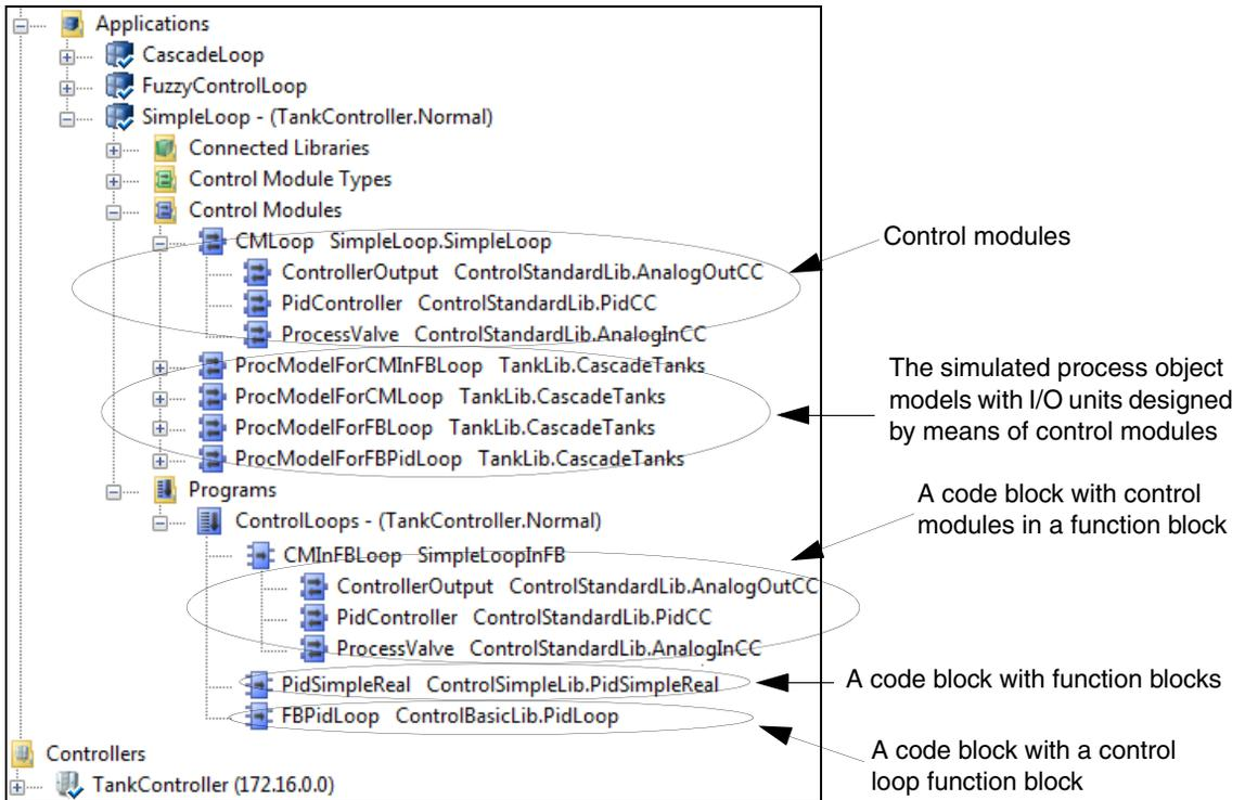
Figure 144. The four methods of designing an application and the simulated process
