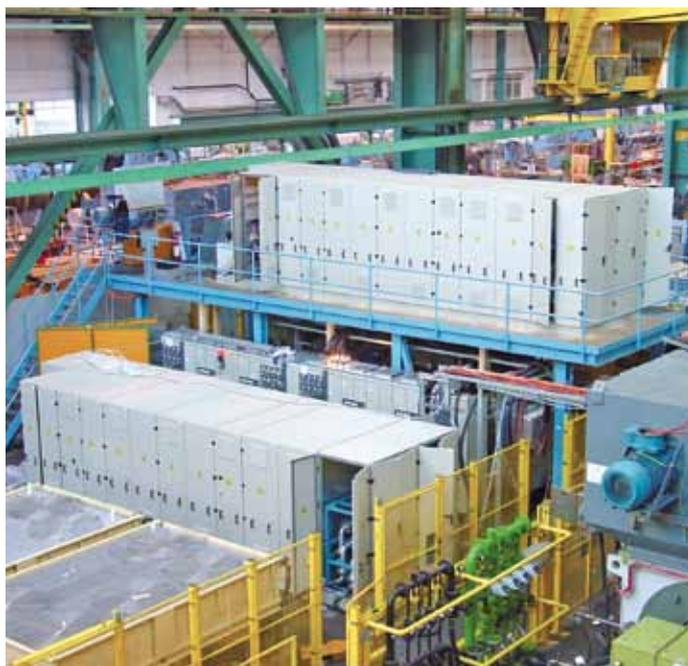
Back-to-Back-Test 8 MW / 3,600 U/min
