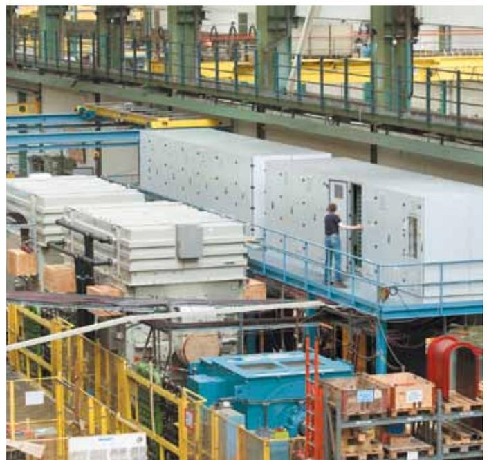
Back-to-Back-Test 48 MW / 3,500 U/min
